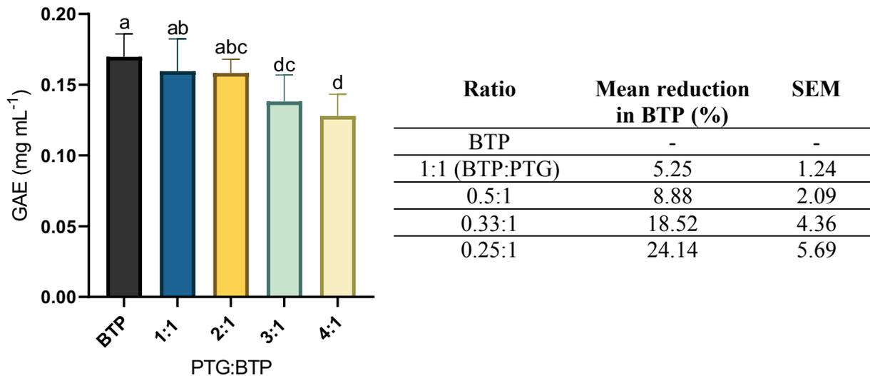
Figure 8. Precipitation of BTP by PTG complexation.
