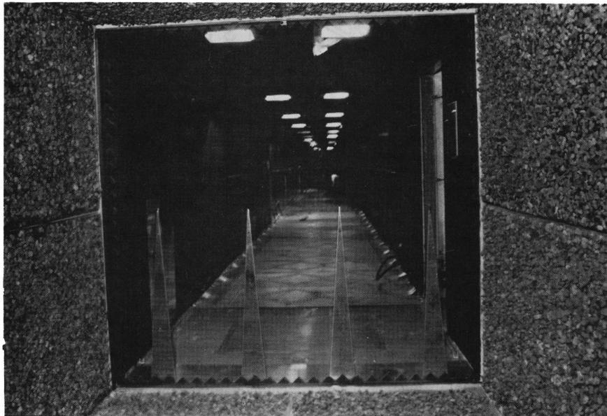
Figure 2-4. Appearance of MWT test-section viewed from entrance.
