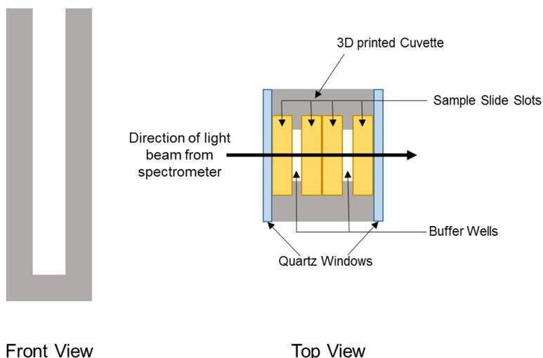
FIGURE V.2: Customized CD cuvette schematic. Adapted from a schematic made by the Latour Group from Clemson University. Slight changes made to width of cuvette to fit into standard sample holder of CD instrument, also cuvette main body made by using a 3D printer.<sup>4</sup>
