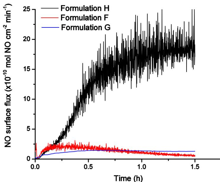
FIGURE II.1: Representative NO release measurements for covalently attached and blended sample methods. Surface flux was determined for films for which contact angles were obtained post-soaking.
