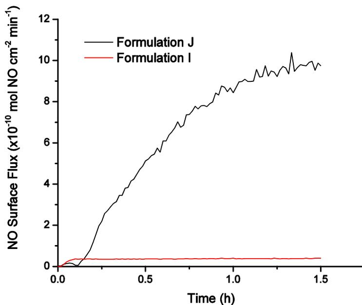
FIGURE II.2: NO release measurements of literature-based blended films. Multi-layered formulation I releases at a steady rate, yet does not release the target NO flux. Formulation J with increased PVC content has potential to release at the target level with continued time.
