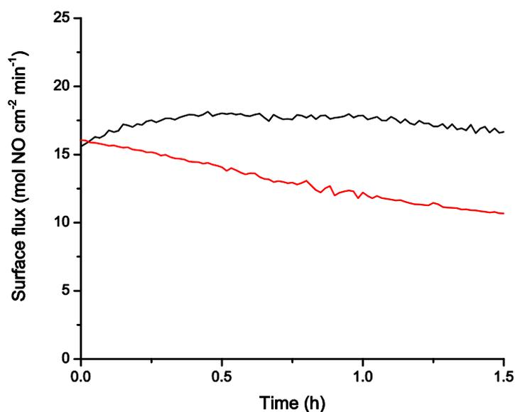
FIGURE III.5: Average surface flux of NO released from 1 wt% (red) and 9.2 wt% (black) composite materials. Shown is 1.5 h of measurement after film has been allowed to release for 1 h to achieve a stable release of NO. Spread in surface flux deviation over release period <5% (n=5).
