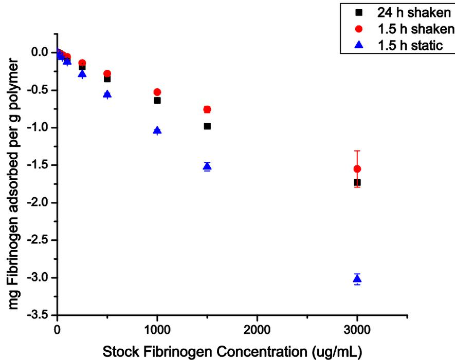
FIGURE IV.3: Comparison of BCA assay results for control film under different reaction conditions: 24 h shaken (blue), 1.5 h shaken (red), 1.5 h static (green). Incubation time has less effect on the values than shaken or static conditions does. Values represented in mean  $\pm$  standard deviation (n=3 for all values).
