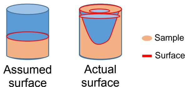
FIGURE II.3: Representation of the expected and actual surface of the multi-layered films used for formulation I. Surfaces were expected to be uniform with a defined surface area, however, the actual films dissolved the wells and became concave with no defined or uniform surface area. These films were made in the break-away wells for NOA experiments.
