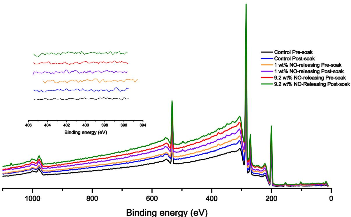
FIGURE III.4: Representative survey scans of material surfaces. Spectra overlay shows no change in surface composition for all samples. Inset is representative high resolution XPS scan for N1s peak. For all samples, peak to noise averages 0-3, indicating no peak for N1s.
