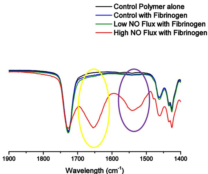
FIGURE V.5: IR spectra of polymer with and without fibrinogen adsorption control (black without and blue with), low NO flux (green), high NO flux (red). Films without fibrinogen adsorption are shown with dashed lines, whereas those with fibrinogen adsorption are solid. The amide I and II peaks are highlighted in yellow and purple, respectively.
