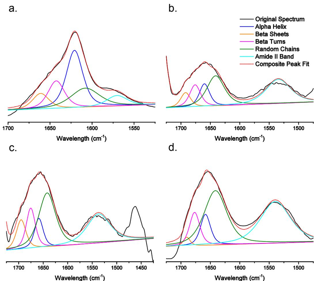
FIGURE V.6: Comparison of native (a) and adsorbed fibrinogen on control (b), low NO flux (c), and high NO flux (d) materials. Adsorbed fibrinogen is on the high NO flux material. Peak deconvolution performed using Thermo Omnic software.
