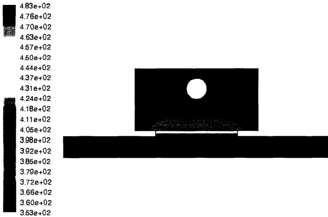
**Figure 5.2: Temperature distribution within the bench top testing apparatus (In Kelvin)**
