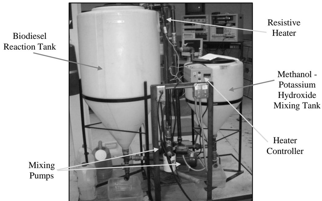
**Figure 3.1 - Large scale biodiesel reactor in the EECL.**
