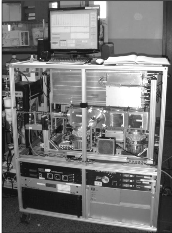
**Figure 2.16 - Aerodyne High-Resolution Time-of-Flight Aerosol Mass Spectrometer.**
