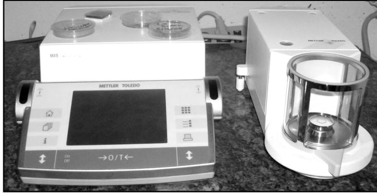
**Figure 2.13 - Microbalance used to weigh the Teflon filters.**
