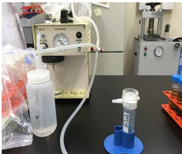
*Figure 6: Filtration system for preparing the exchangeable fraction samples.*
