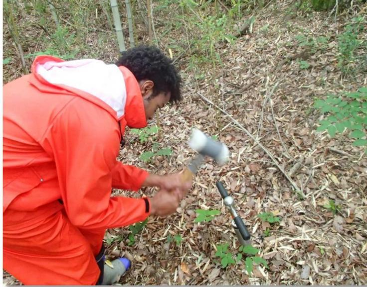
Figure 1: The soil core sampling equipment is used here to collect a virtually undisturbed soil core sample for environmental study.
