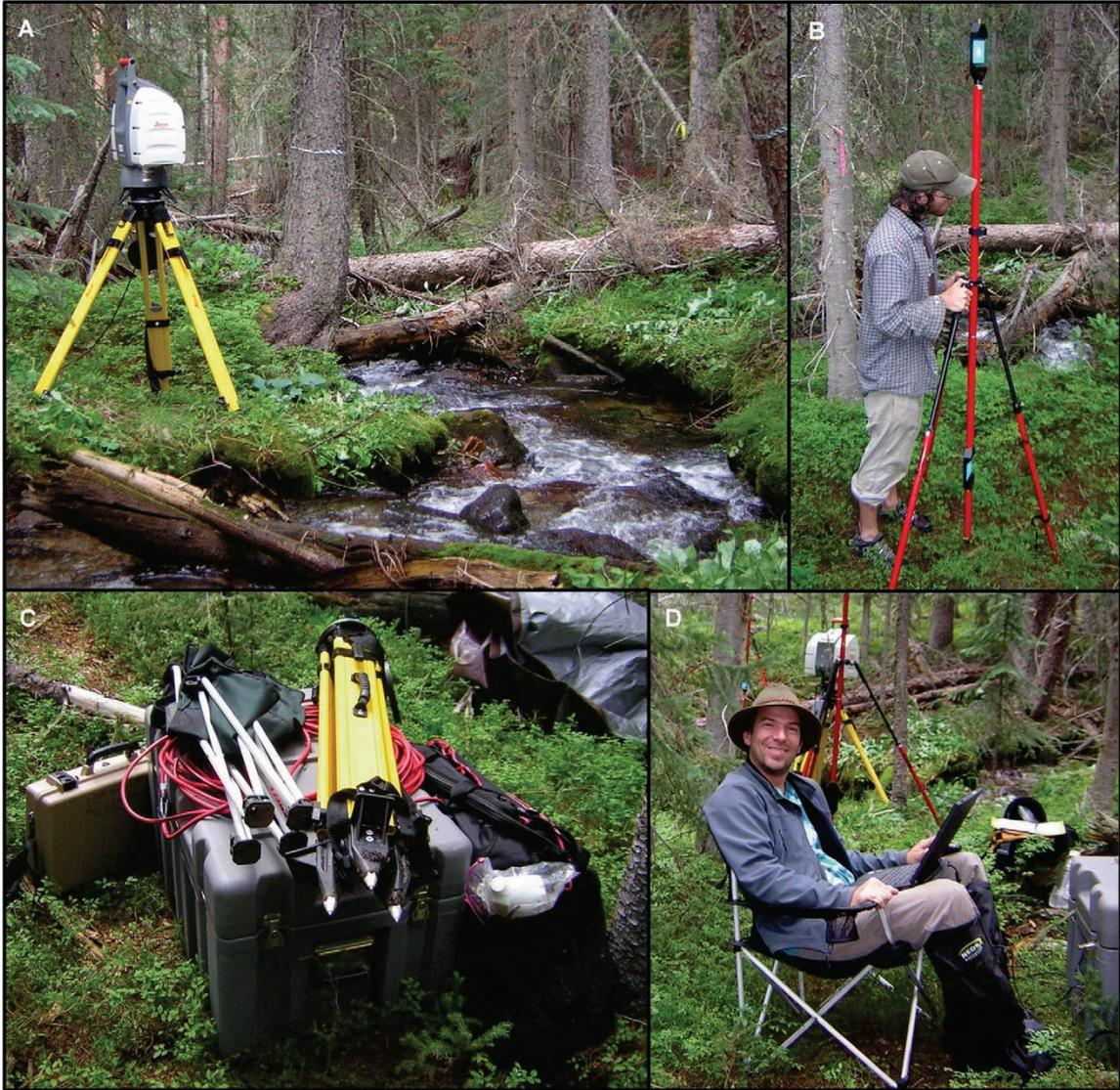
A: LiDAR scanner, set up on reach ESL-9
