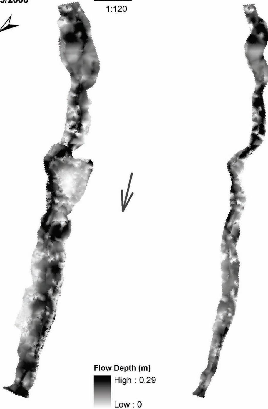
Figure D-29: Depth variability for mid flow, reach FC-1 (7/23/2008).
