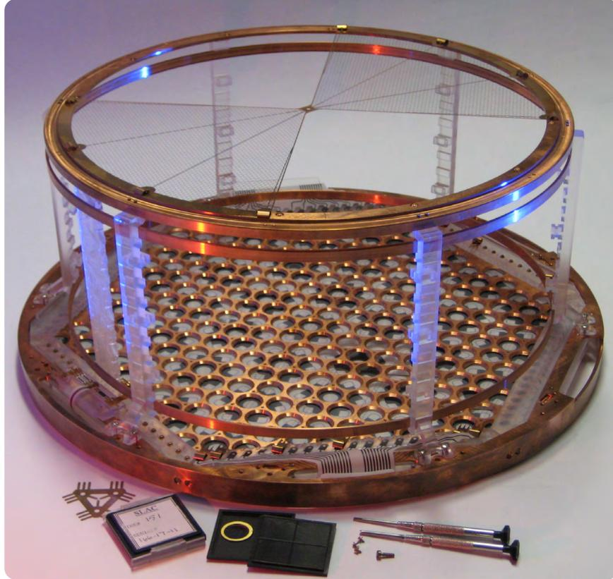
**Figure 1.4:** Picture of half of the EXO 200 TPC before installation. The top part is the cathode grid, and the anode wires are in the bottom part. The APD's, which are installed in the holes at the bottom, are not shown in this picture.
