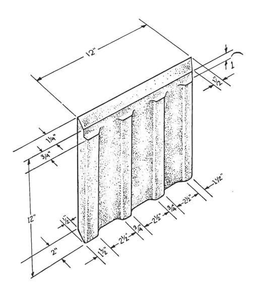
Figure 3. Roofblok Ballast Block
