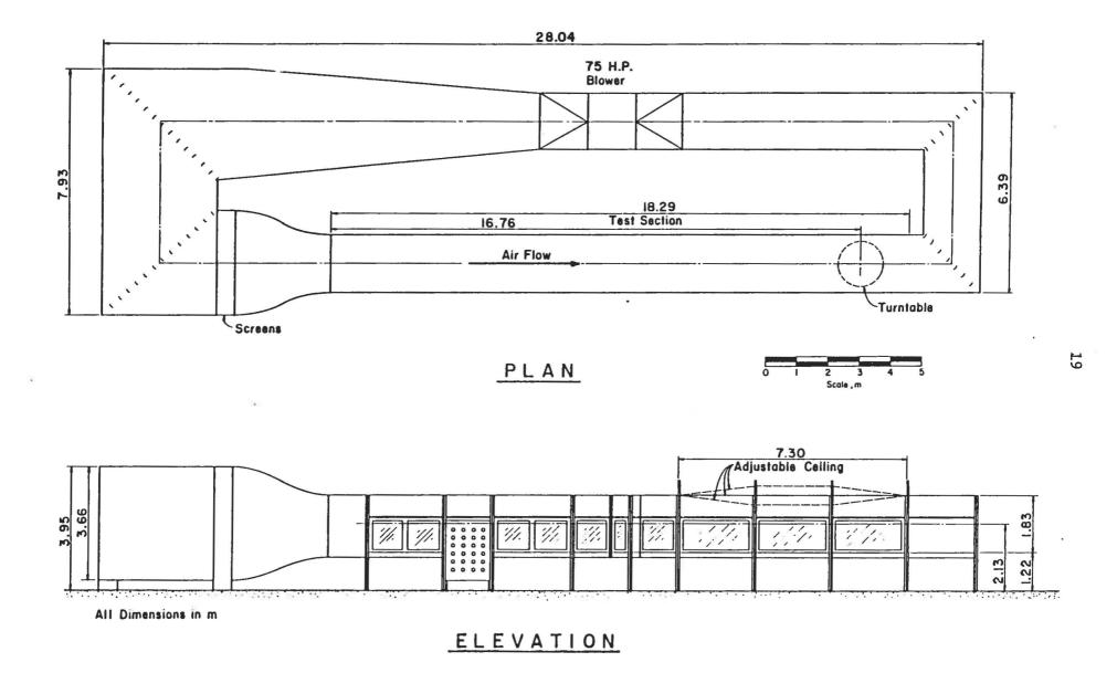
Figure 2. Industrial Aerodynamics Wind Tunnel
