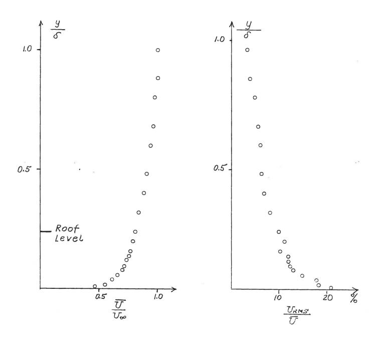
Figure 7. Mean Wind Speed and Turbulence Intensity Profiles
