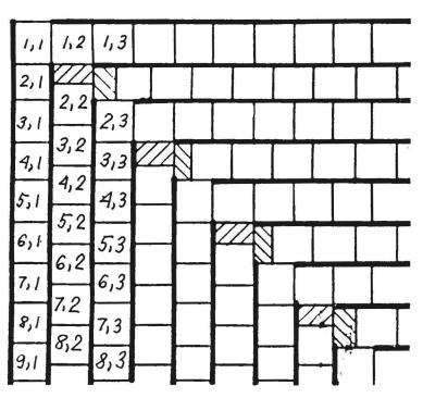
Figure 17. Identification of Ballast Blocks
