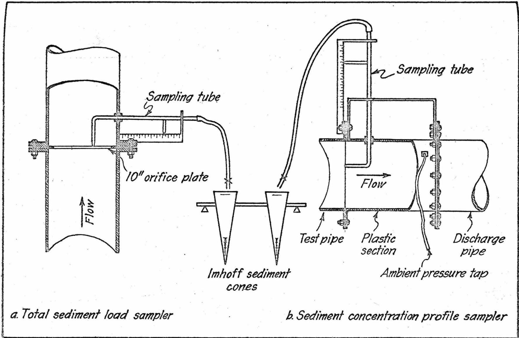
Fig. ■ Schematic diagram of sampling equipment.
