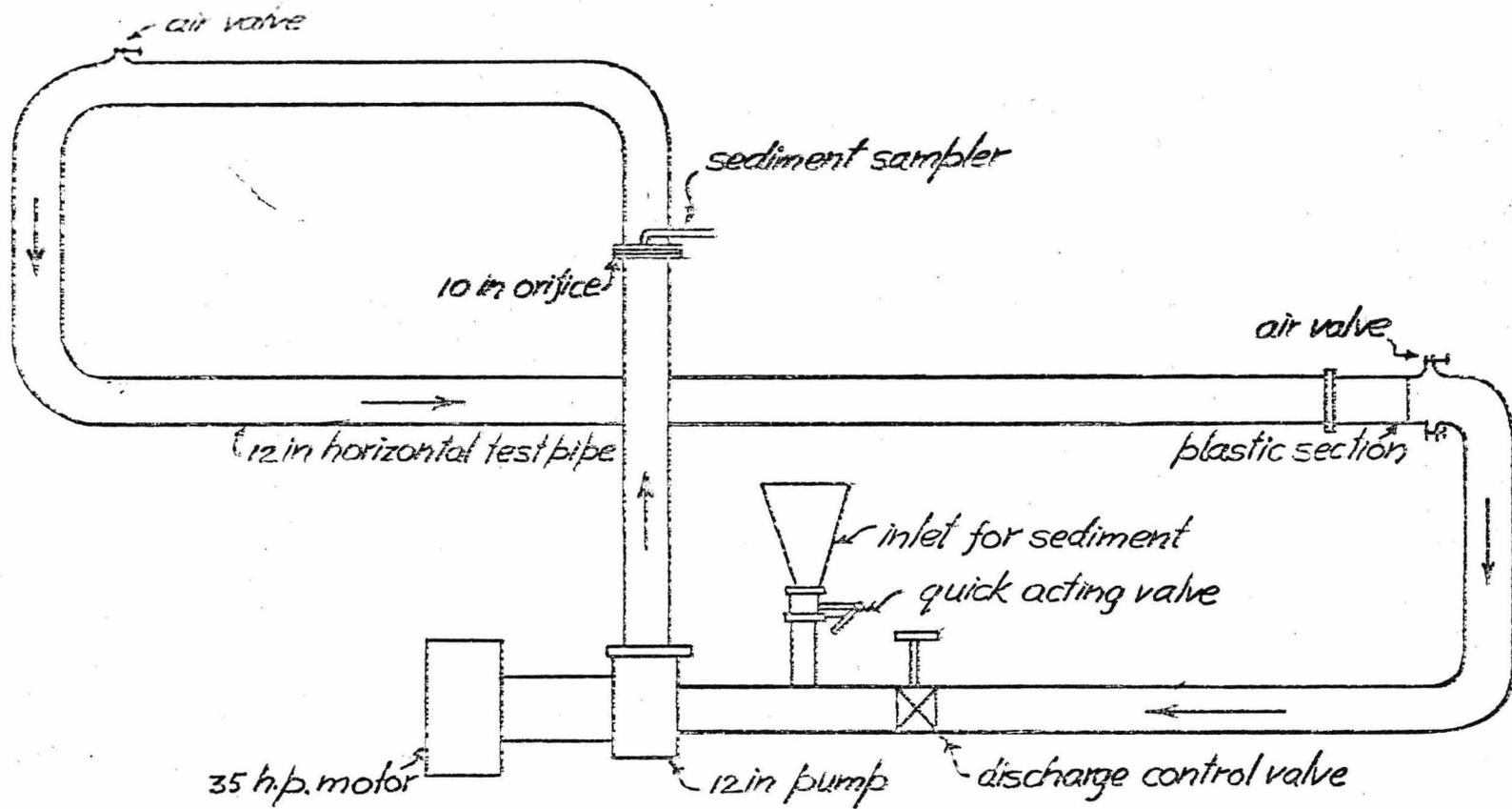
Fig.3 General lay-out of the recirculation system.
