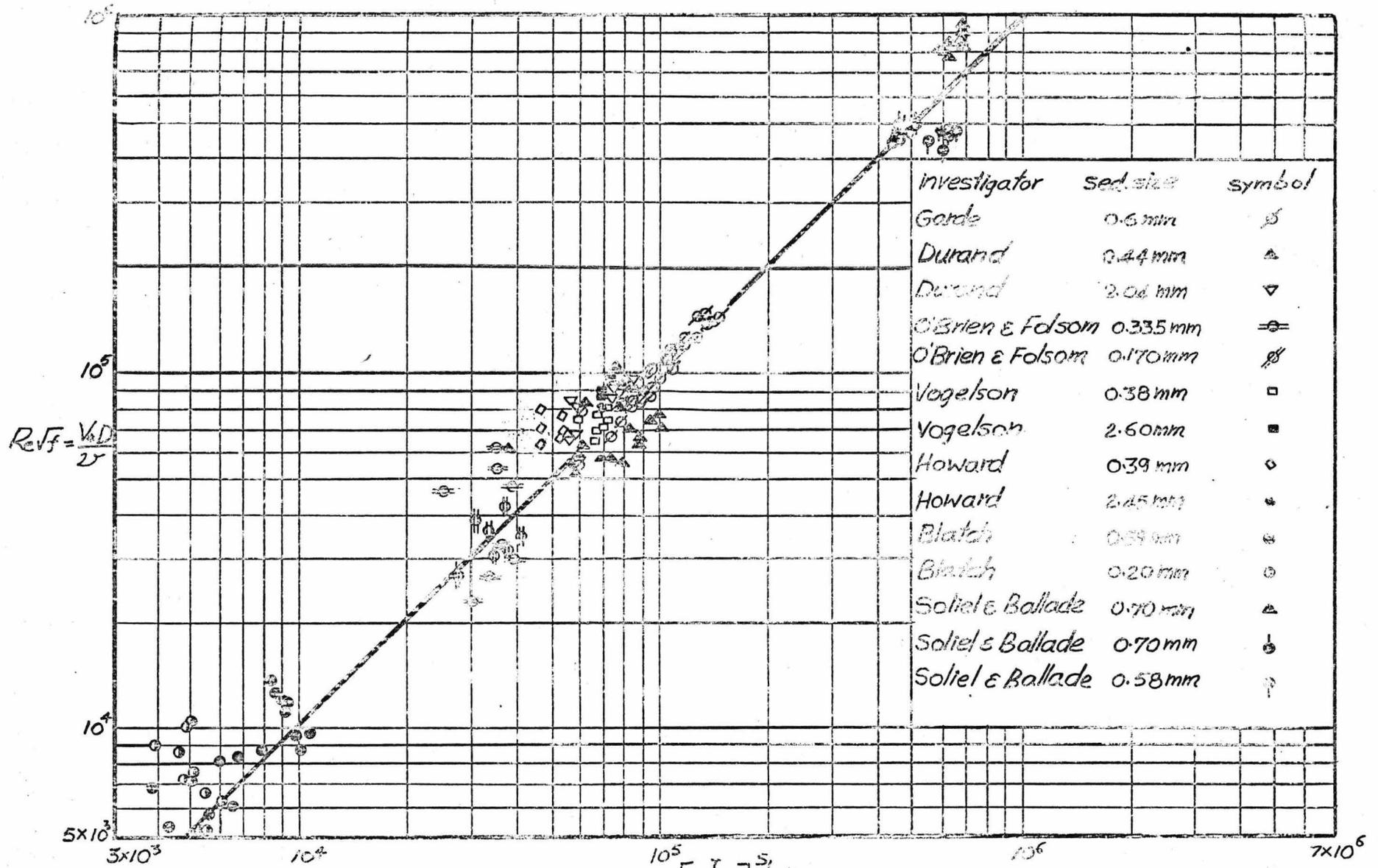
Fig. 1 Variation of  $Re\sqrt{f}$  with  $\left[\frac{L}{d}\right] S_1 C_1^{1/3}$  for smooth boundary
