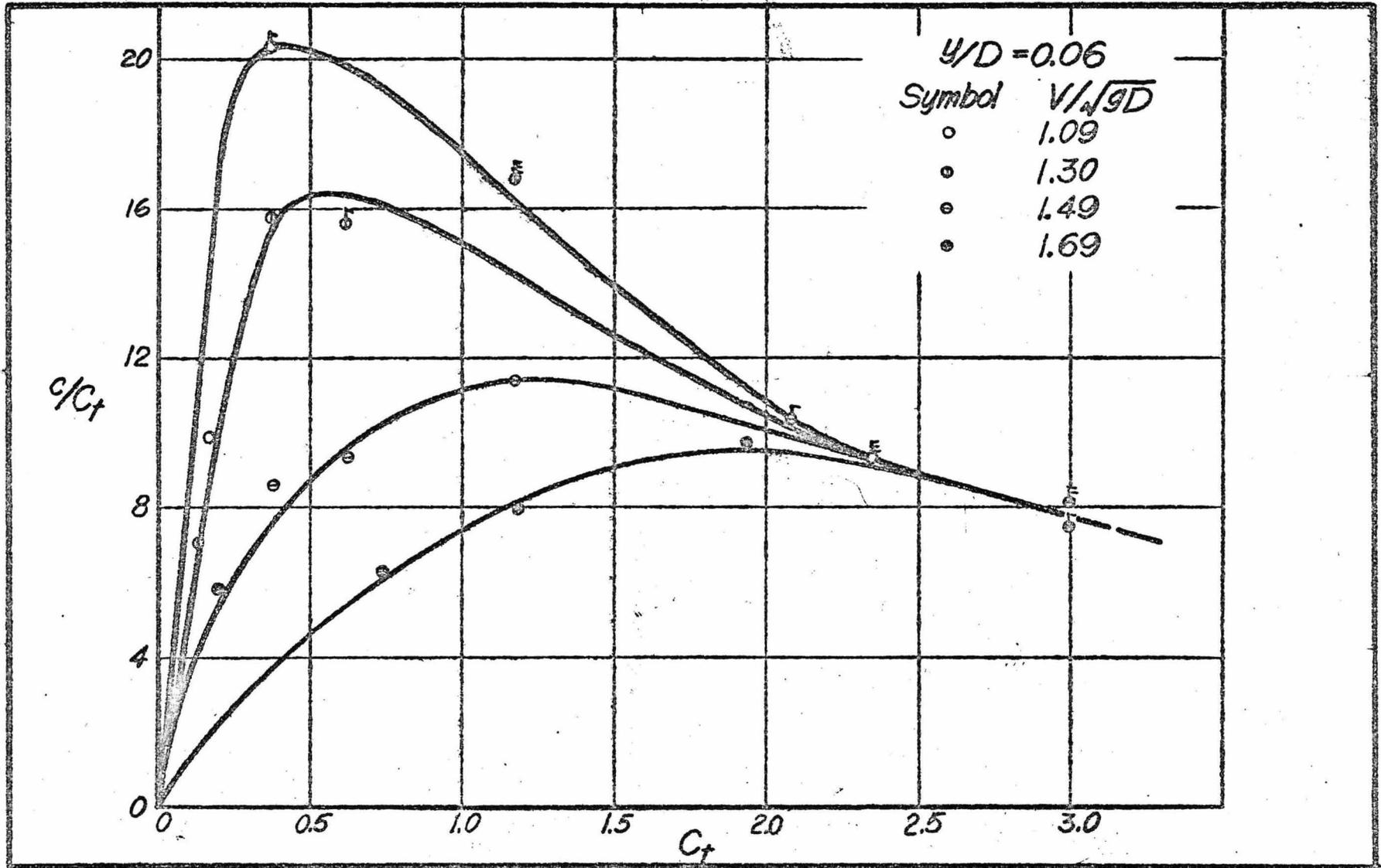
Fig. 23 Absolute criterion for incipient deposition—12-in. smooth pipe.
