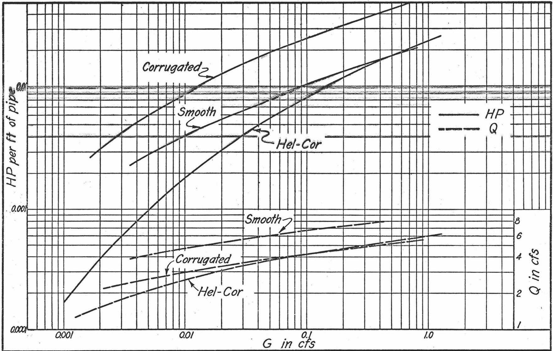
Fig. 1 Variation of horsepower and discharge of mixture with sediment discharge.
