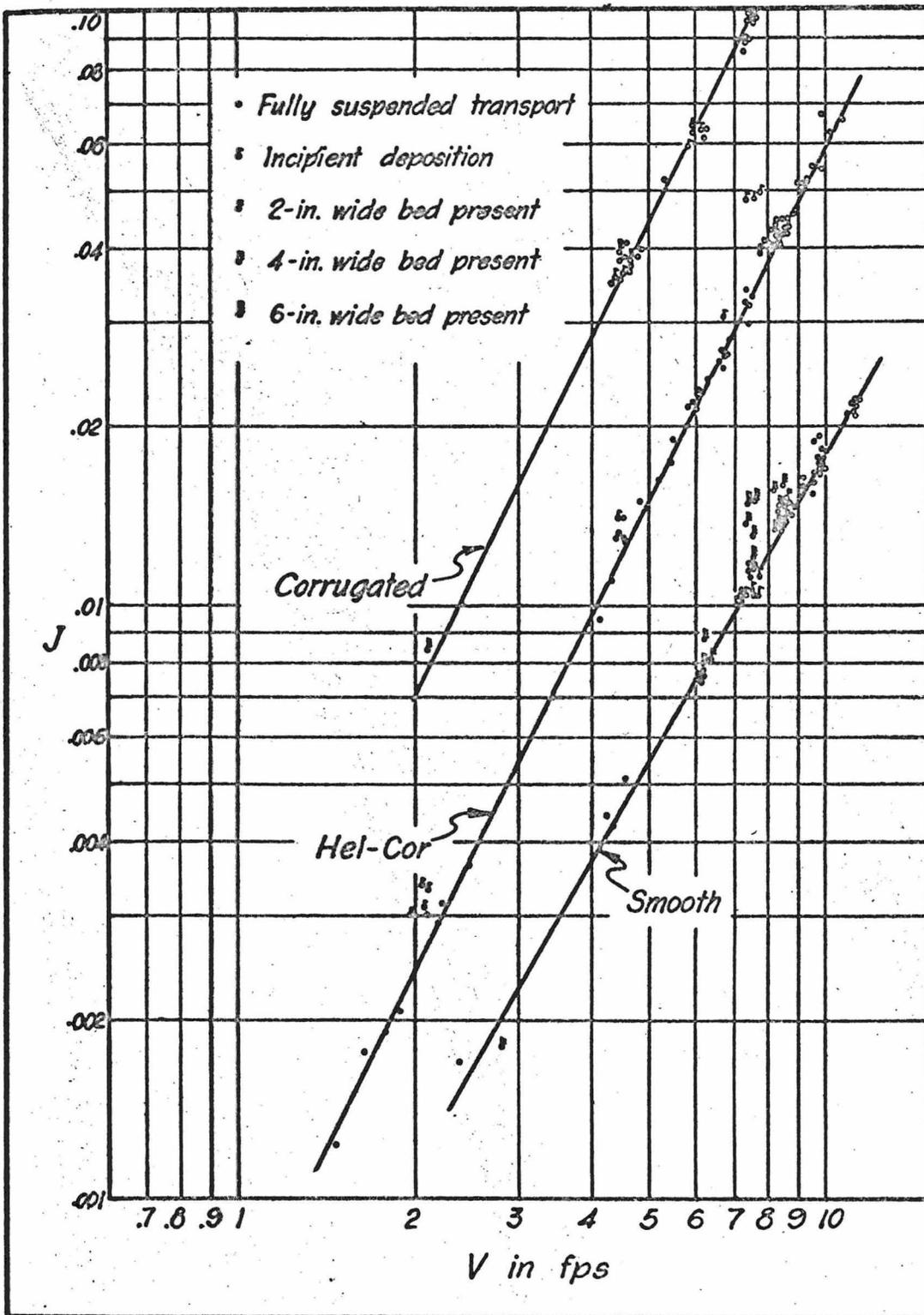
Fig. 5 Variation of hydraulic gradient with velocity and concentration.
