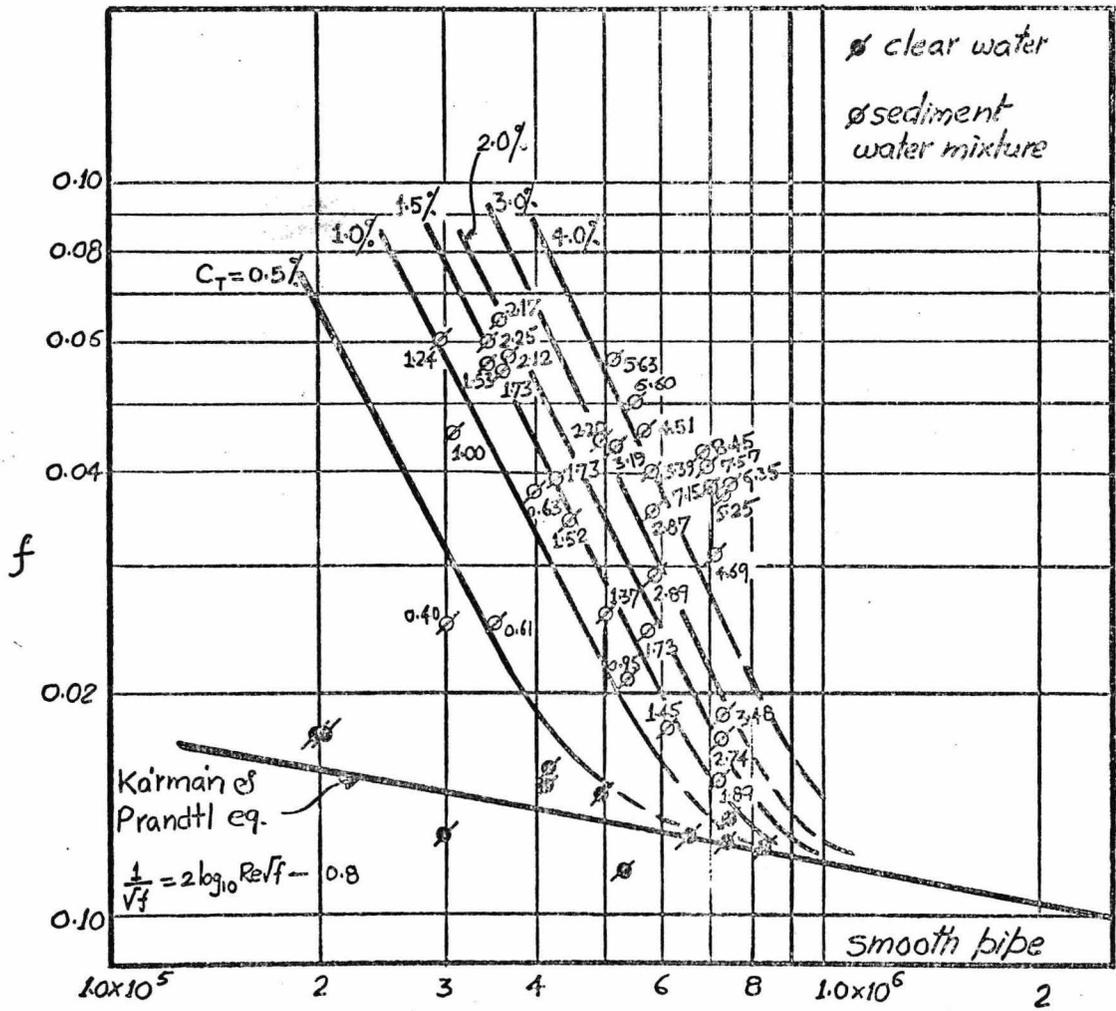
Fig. 9 Variation of  $f$  with  $Re$  and  $G_T$  for smooth and standard corrugated pipes.
