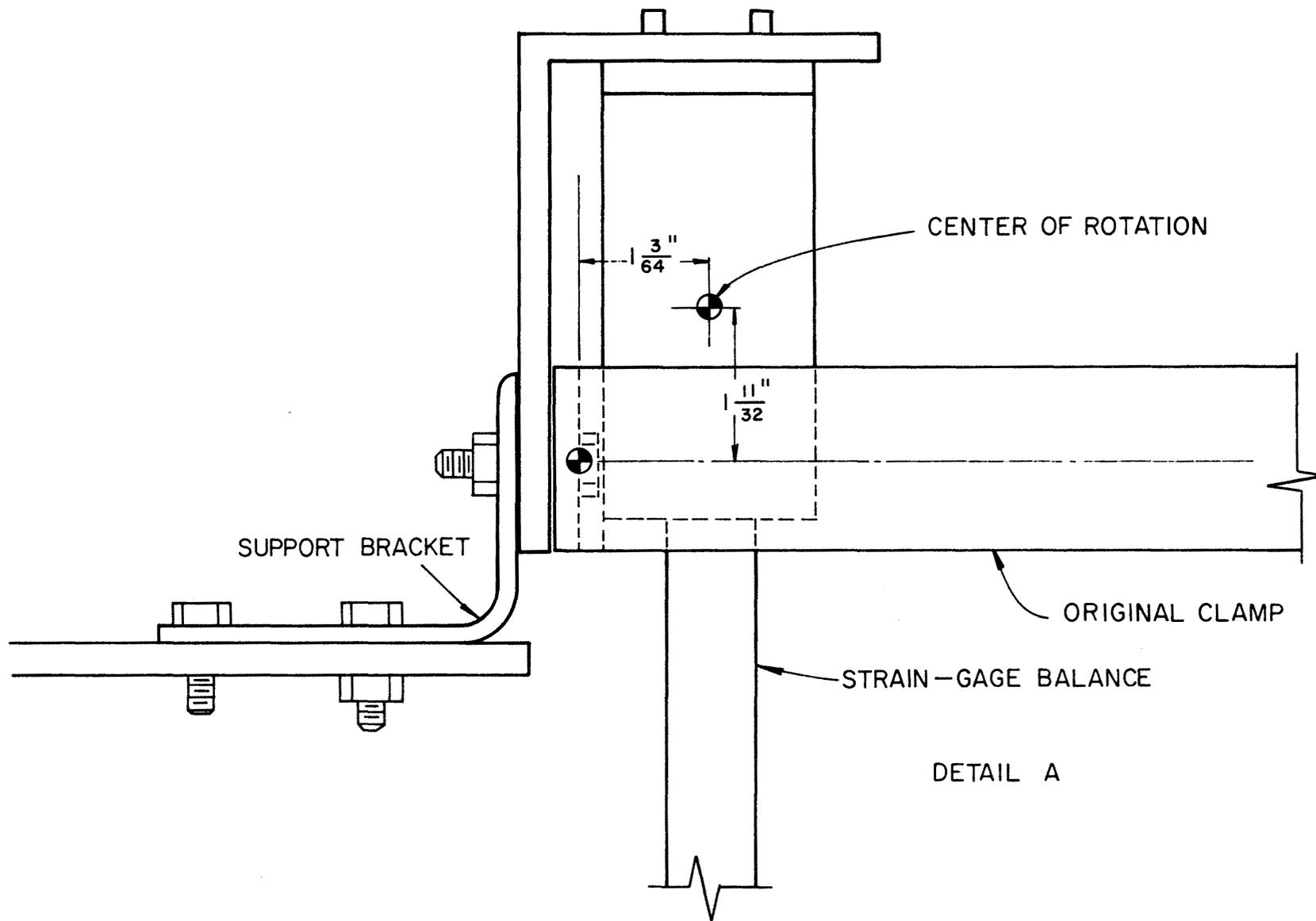
Figure 4 Detail A for the center of rotation
