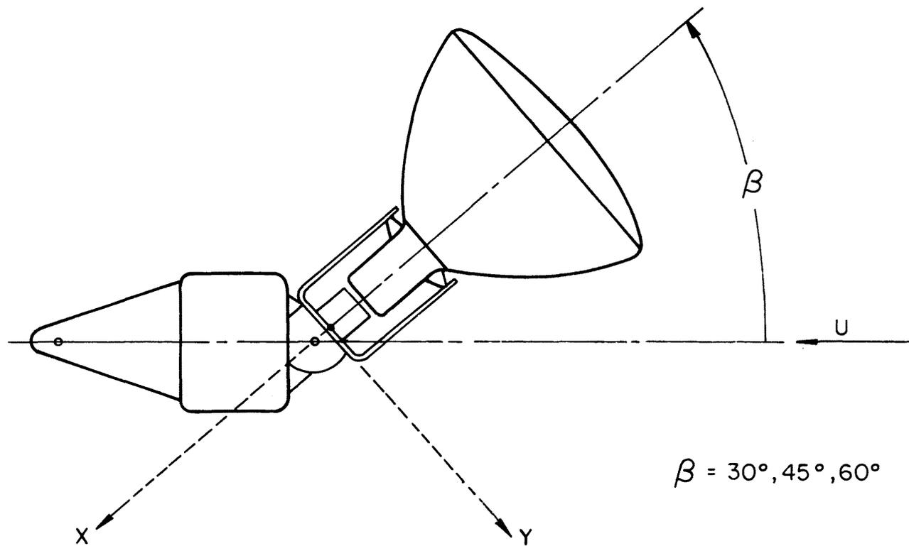
Figure 6 Orientation of angle  $\beta$  with axes of reference
