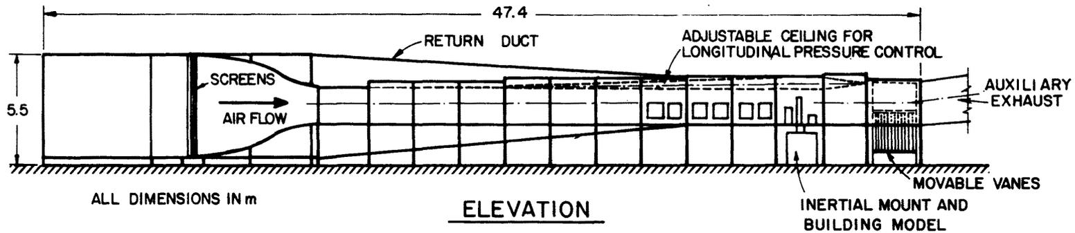
Figure 3 Meteorological Wind Tunnel
