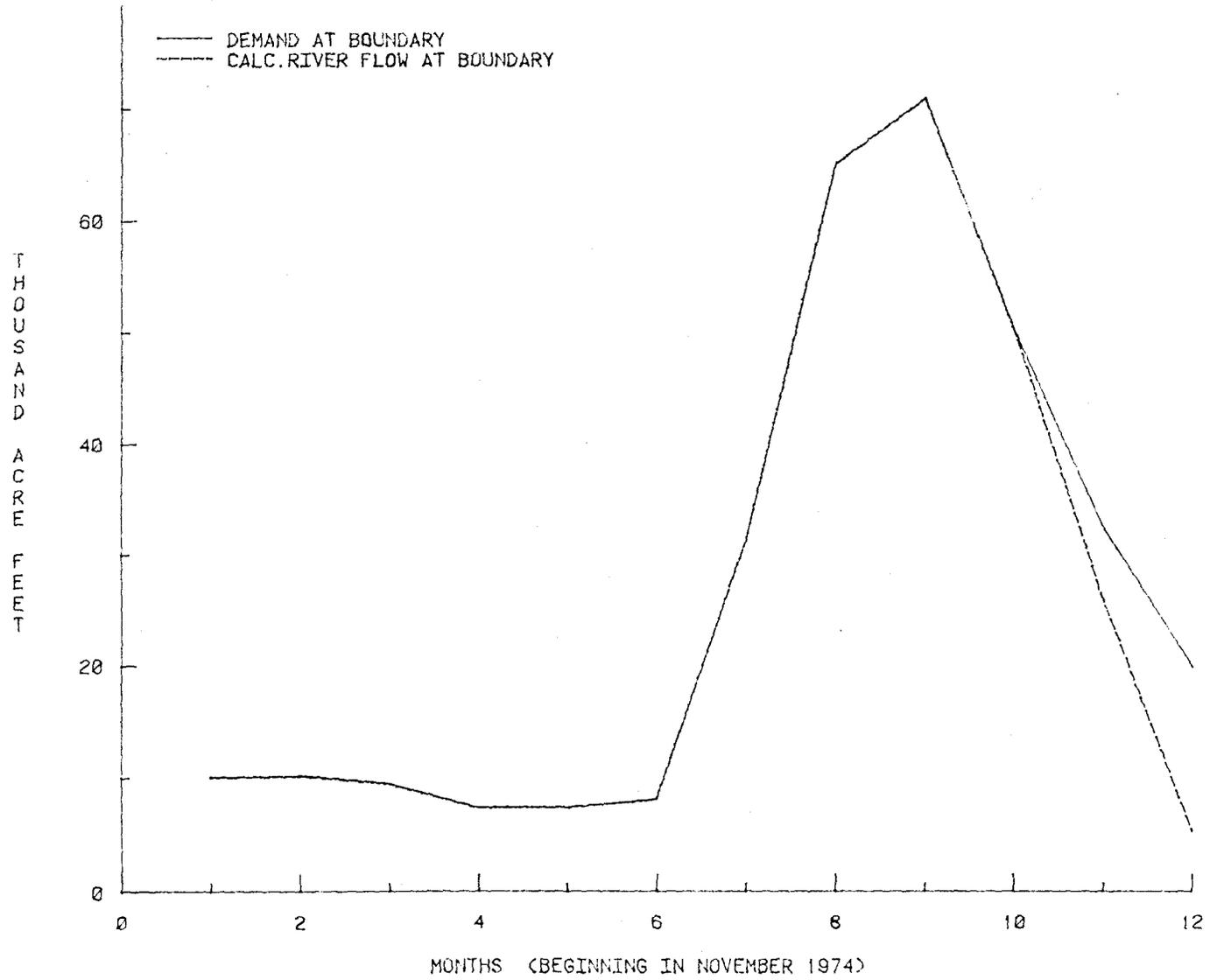
Figure 15. Calibration for Rawhide Project Irrigation Year 1975
