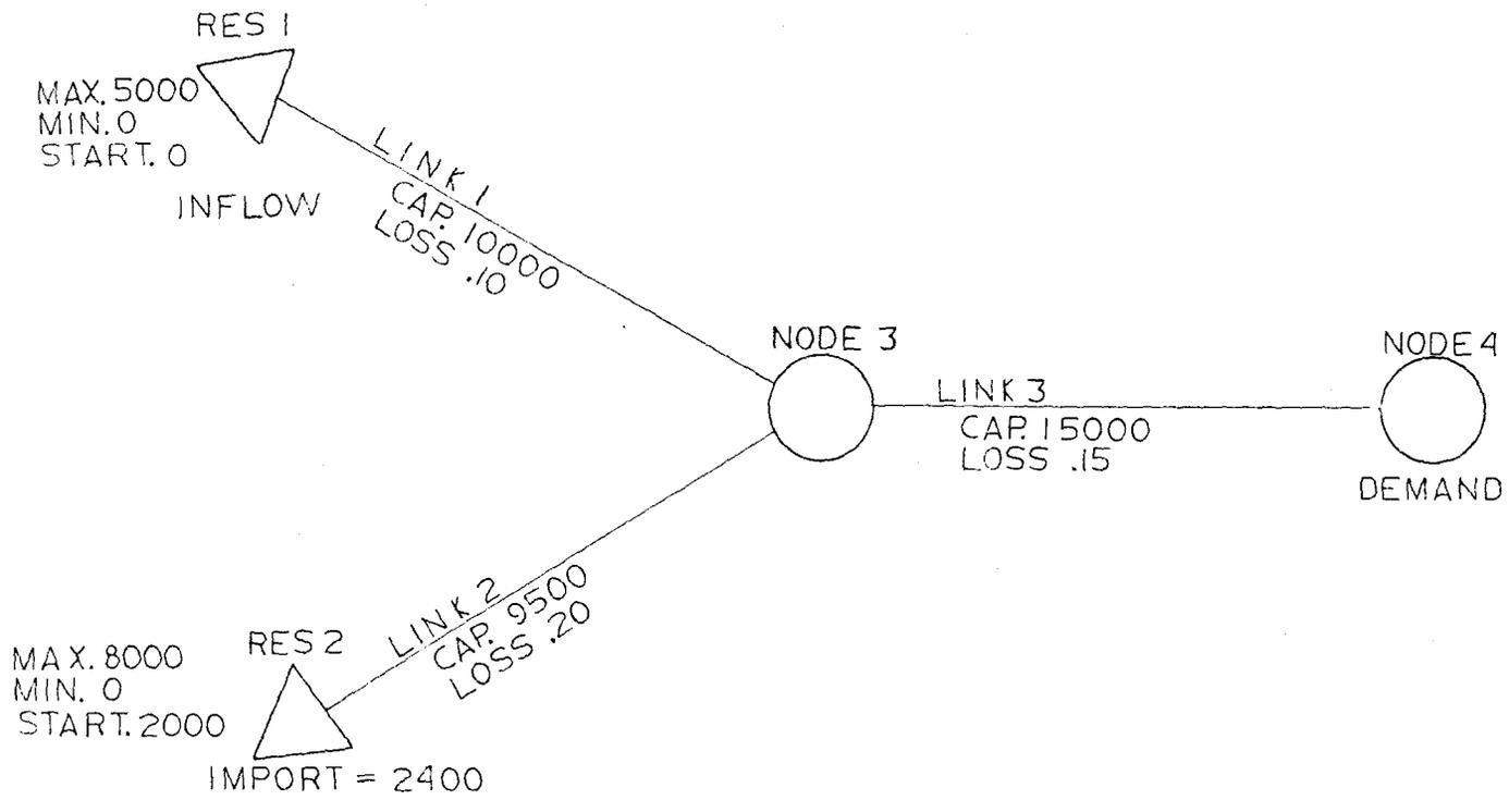
Figure 3. Example Node-Link Configuration
