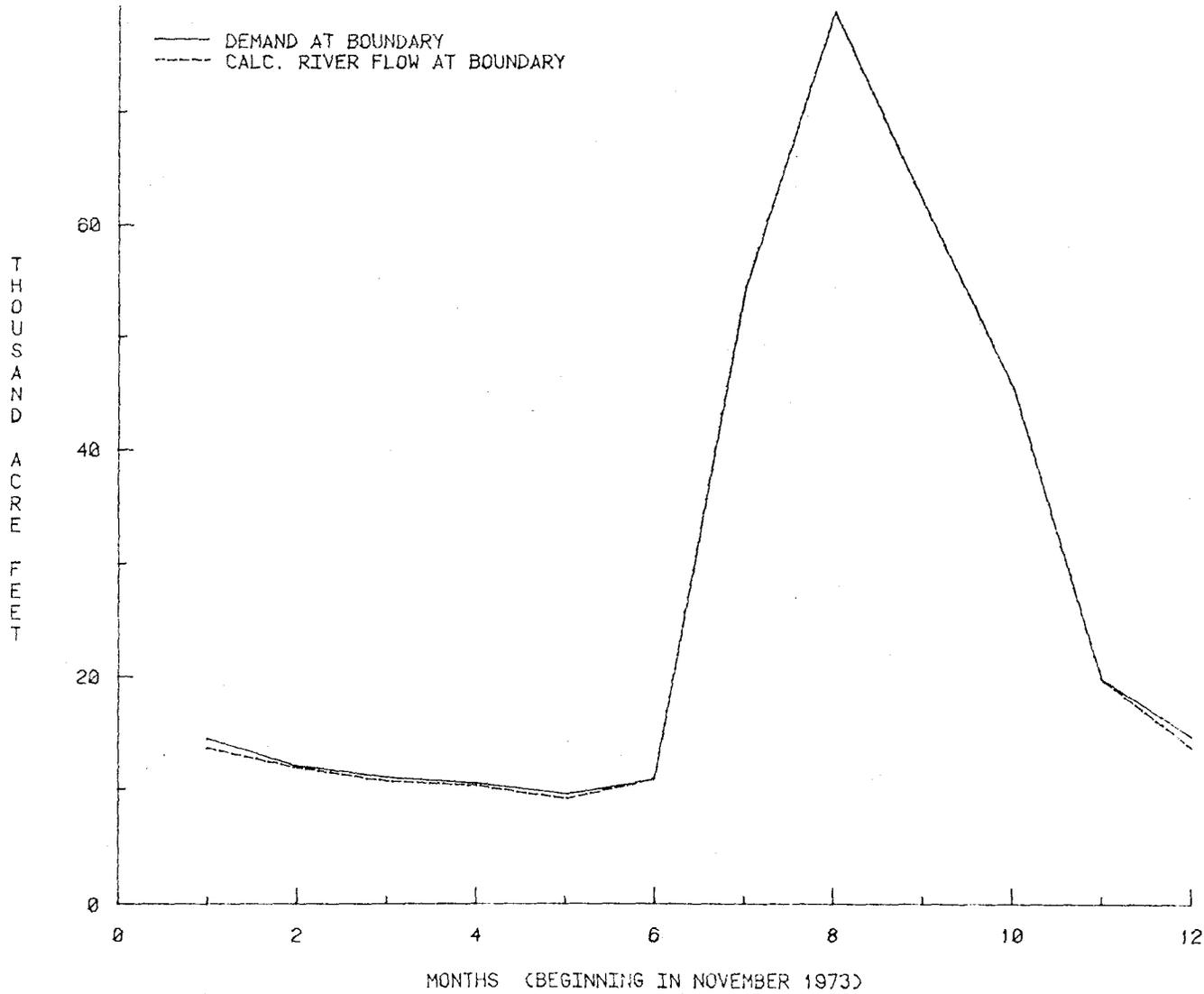
Figure 13. Calibration for Rawhide Project Irrigation Year 1974
