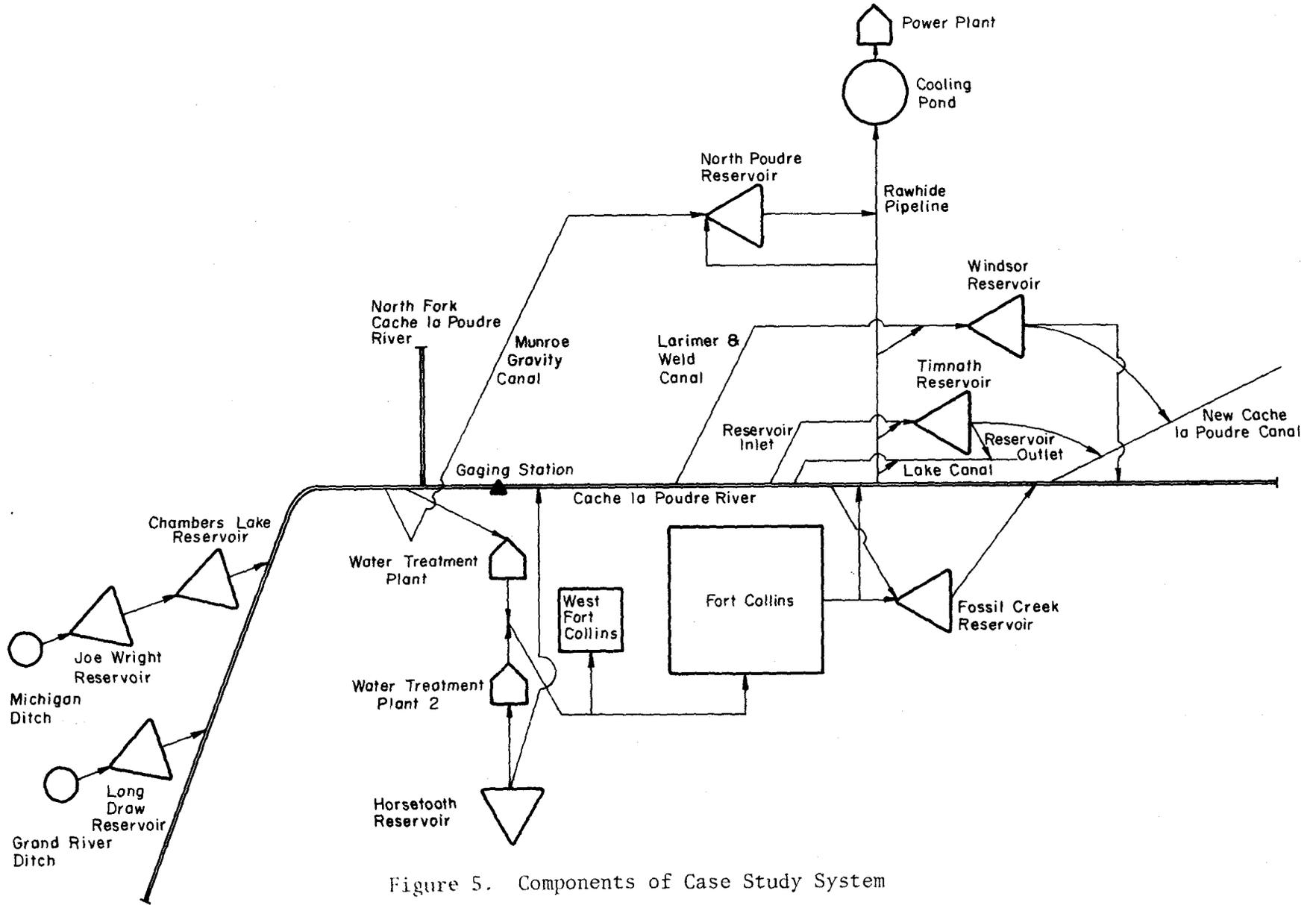
Figure 5. Components of Case Study System
