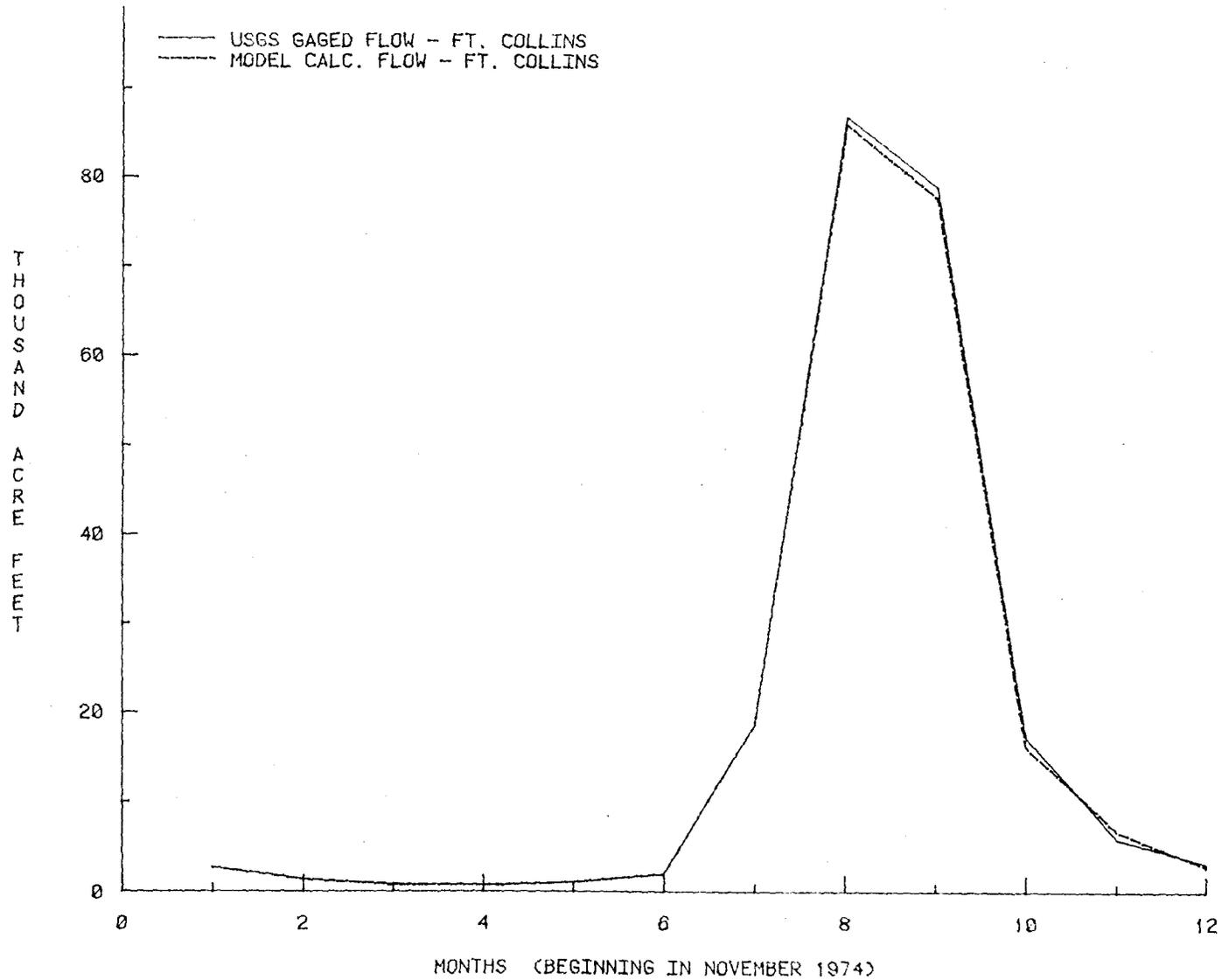
Figure 14. Calibration for Rawhide Project Irrigation Year 1975
