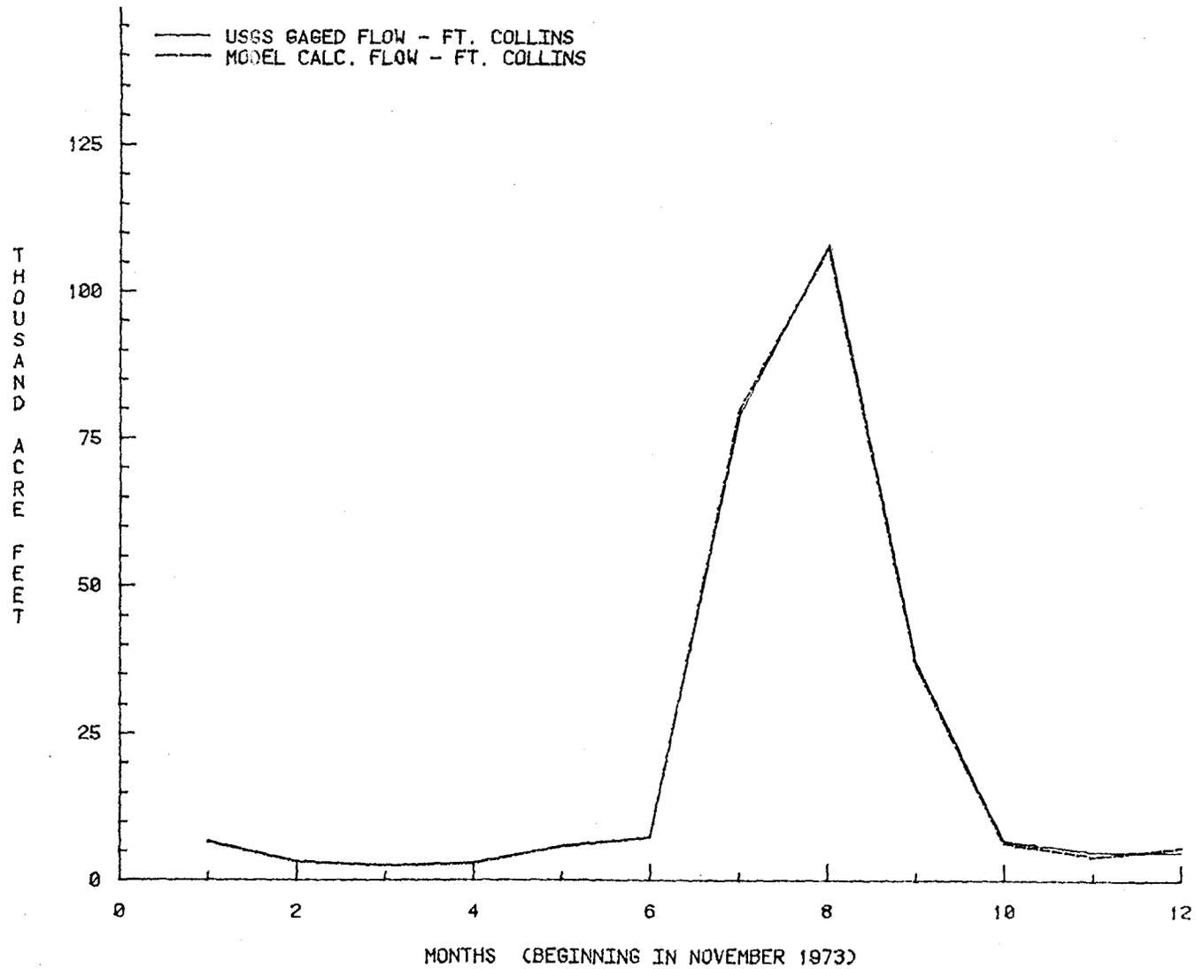
Figure 12. Calibration for Rawhide Project Irrigation Year 1974
