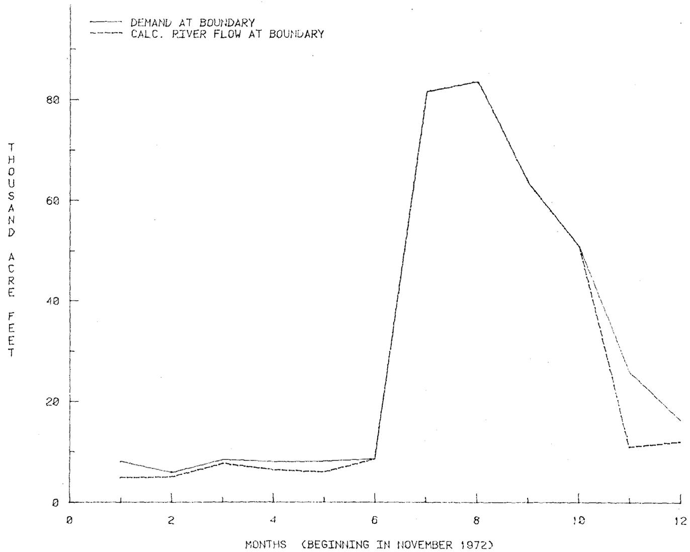
Figure 11. Calibration for Rawhide Project Irrigation Year 1973
