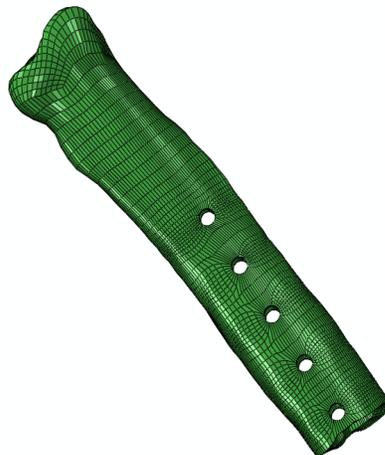
Figure 34-Radius with holes created in TrueGrid for insertion of proximal screws.
