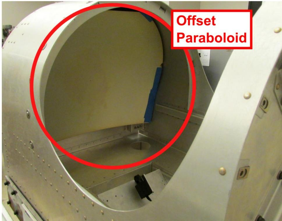
**Figure 2-4: Offset paraboloid reflector mounted in the chassis**
