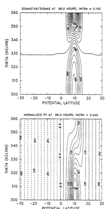
Figure 6.3: Results for T=4 days. (a) Isolines of  $\sigma^*/\sigma_0$  (i.e., potential pseudodensity measured in units of  $\sigma_0$ ) in  $(\Phi,\Theta)$  space. (b) Isolines of  $\sigma_0 P/(2\Omega)$  (i.e., potential vorticity measured in units of  $2\Omega/\sigma_0$ ).
