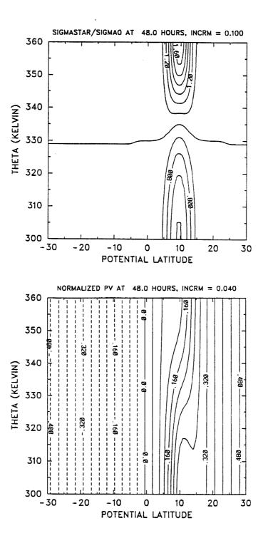
Figure 6.1: Results for T=2 days. (a) Isolines of  $\sigma^*/\sigma_0$  (i.e., potential pseudodensity measured in units of  $\sigma_0$ ) in  $(\Phi,\Theta)$  space. Note that the convection of the ITCZ generates a lower tropospheric layer of high potential vorticity and an upper tropospheric layer of low potential vorticity. (b) Isolines of  $\sigma_0 P/(2\Omega)$  (i.e., potential vorticity measured in units of  $2\Omega/\sigma_0$ ).
