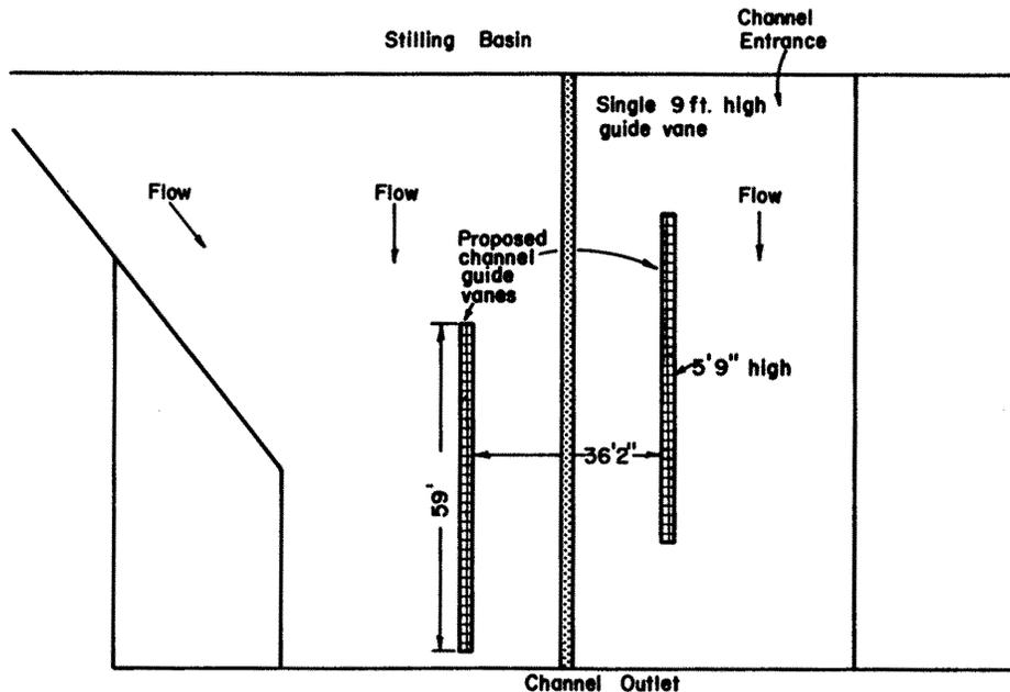
Figure 8 - Plan View of Outflow Channel with Recommended Guide Vanes
