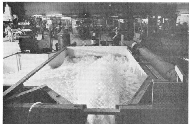
Figure 10f - Flow conditions in recommended flip bucket plunge pool
