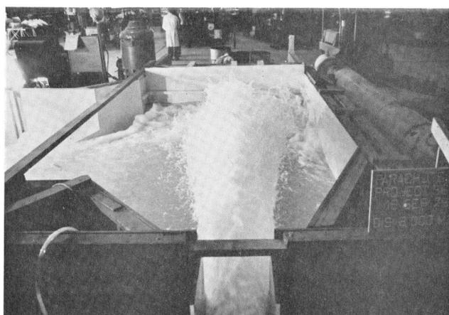
Figure 10b - Flow conditions in recommended flip bucket plunge pool stilling basin and outlet channel entrance, 8,000 cfs
