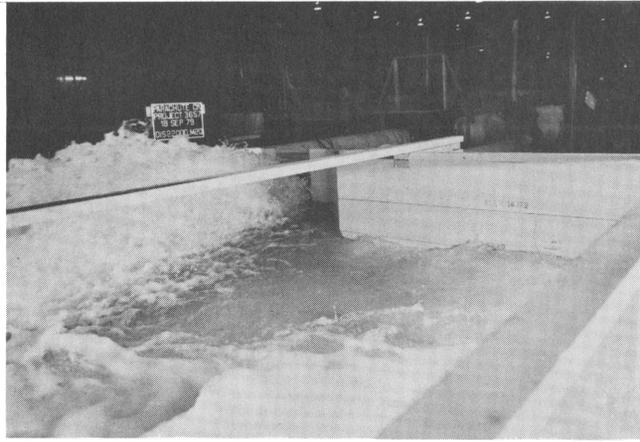
Figure 11 - Waves near outlet channel entrance
