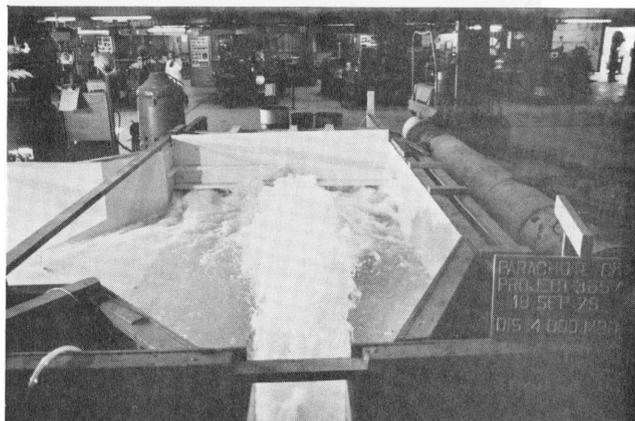
Figure 10a - Flow conditions in recommended flip bucket plunge pool stilling basin and outlet channel entrance, 4,000 cfs
