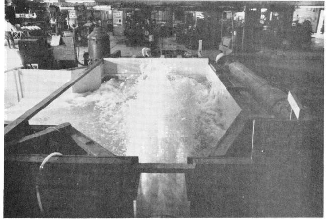
Figure 10d - Flow conditions in recommended flip bucekt plunge pool
