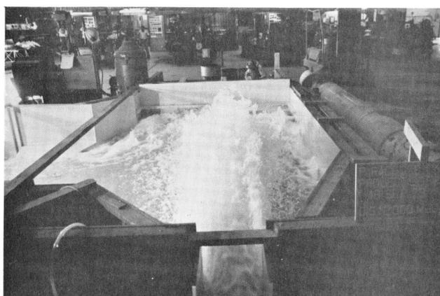
Figure 10c - Flow conditions in recommended flip bucket plunge pool stilling basin and outlet channel entrance, 12,000 cfs
