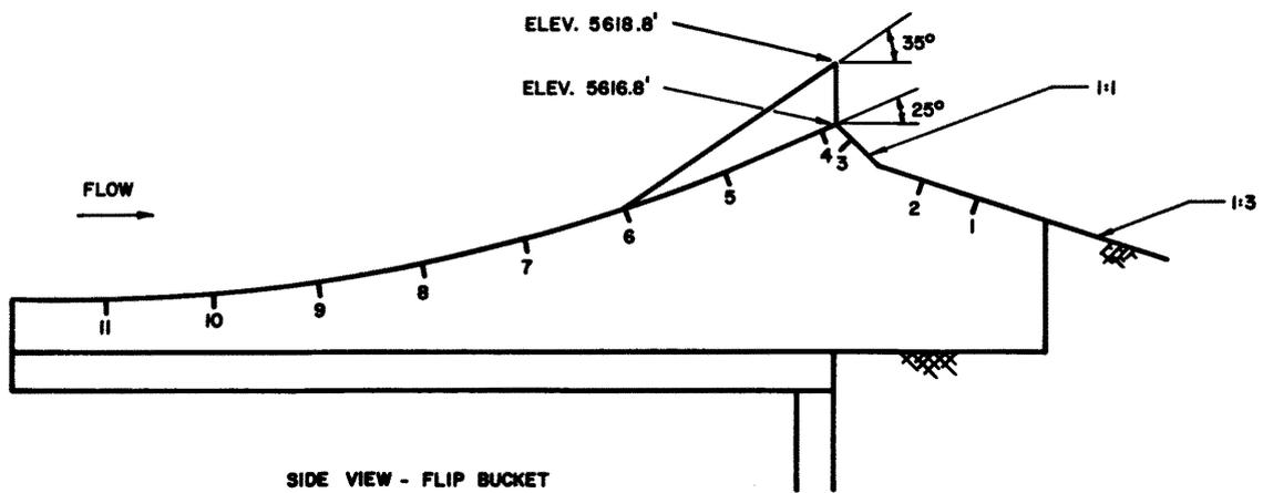
Figure 5 - Piezometer Locations in Flip Bucket
