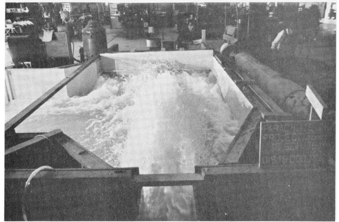
Figure 10e - Flow conditions in recommended flip bucket plunge pool
