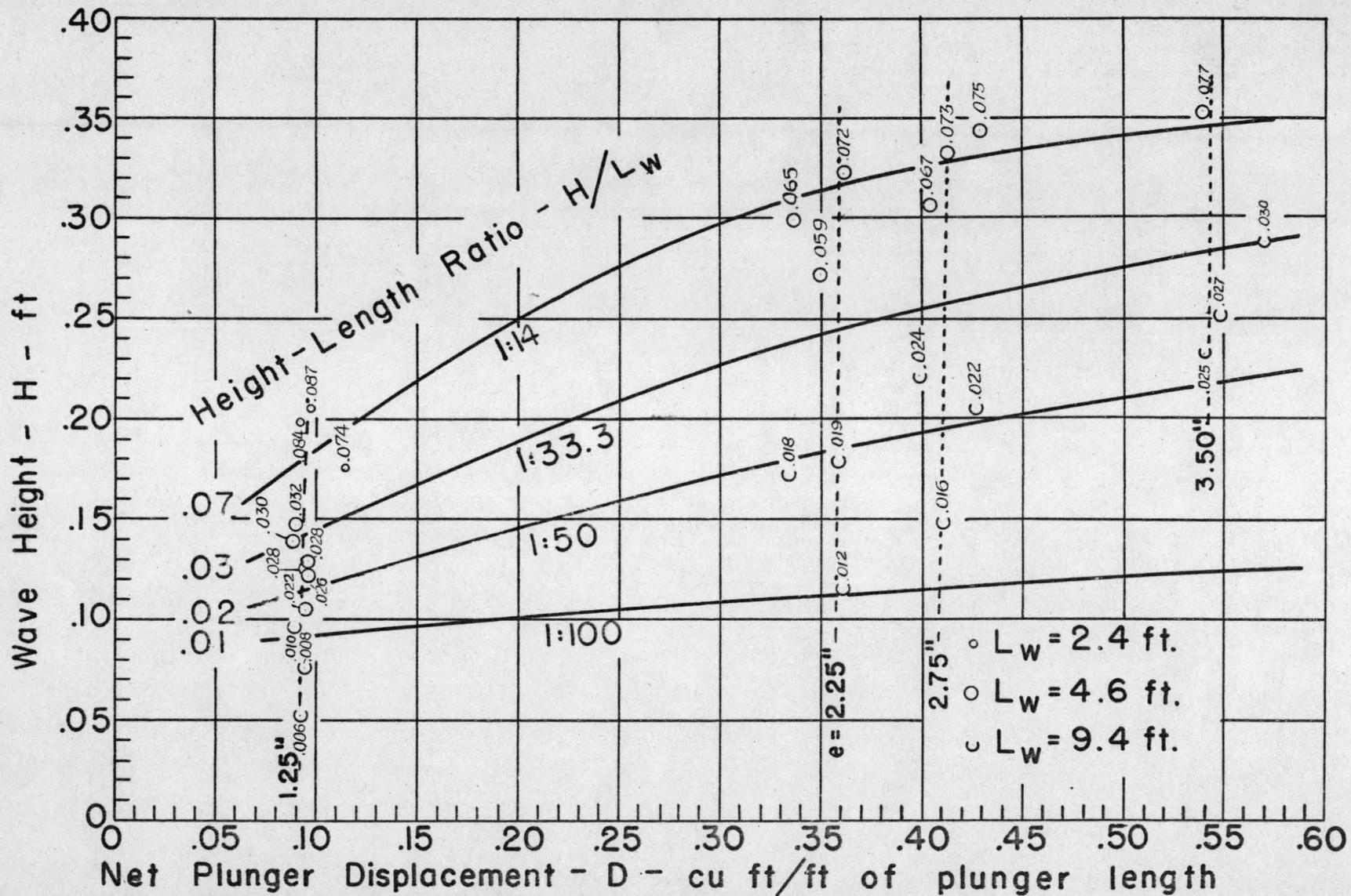
Fig. 3-WAVE GENERATOR PERFORMANCE
