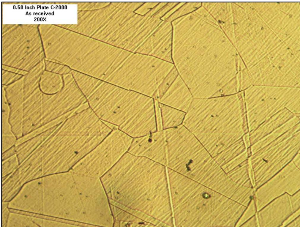
*Figure 34 C-2000 0.50 inch Plate - As Received*
