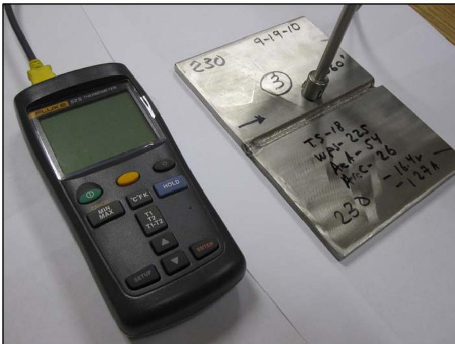
*Figure 9 Fluke Thermometer and Probe*
