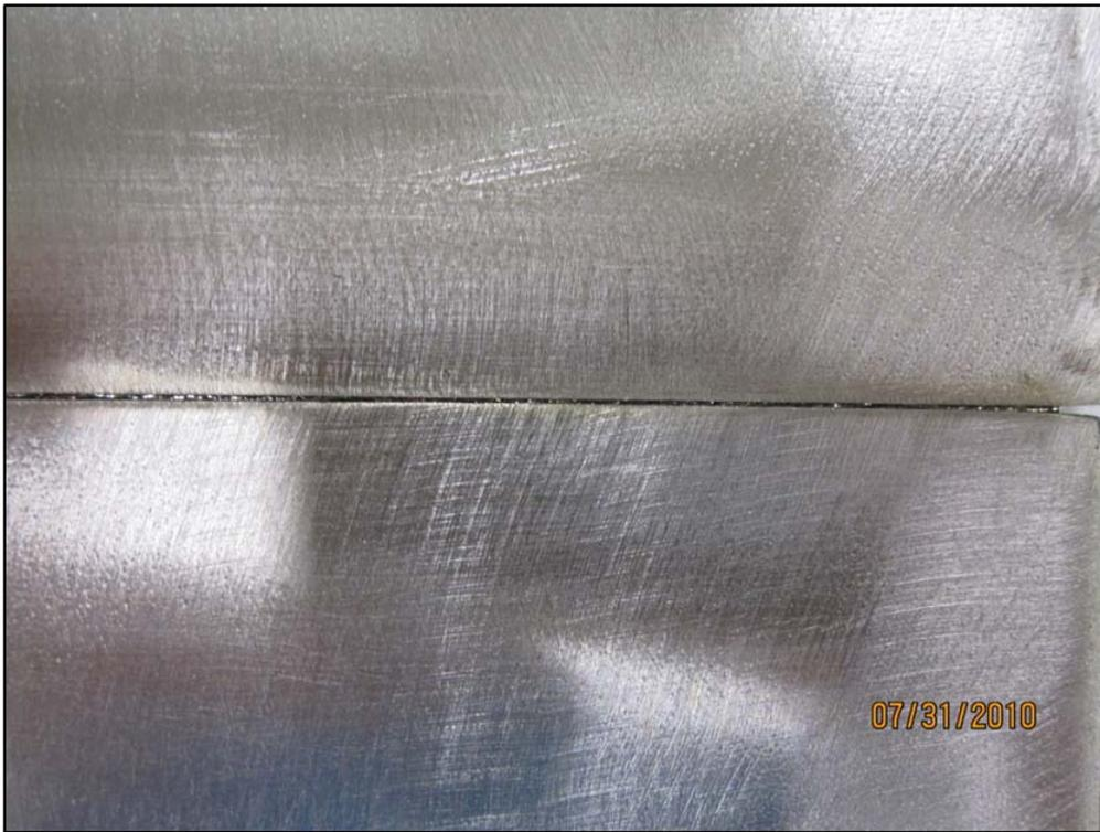
*Figure 20 B-3 Sample 30 - Root Pass -Lack of Penetration*
