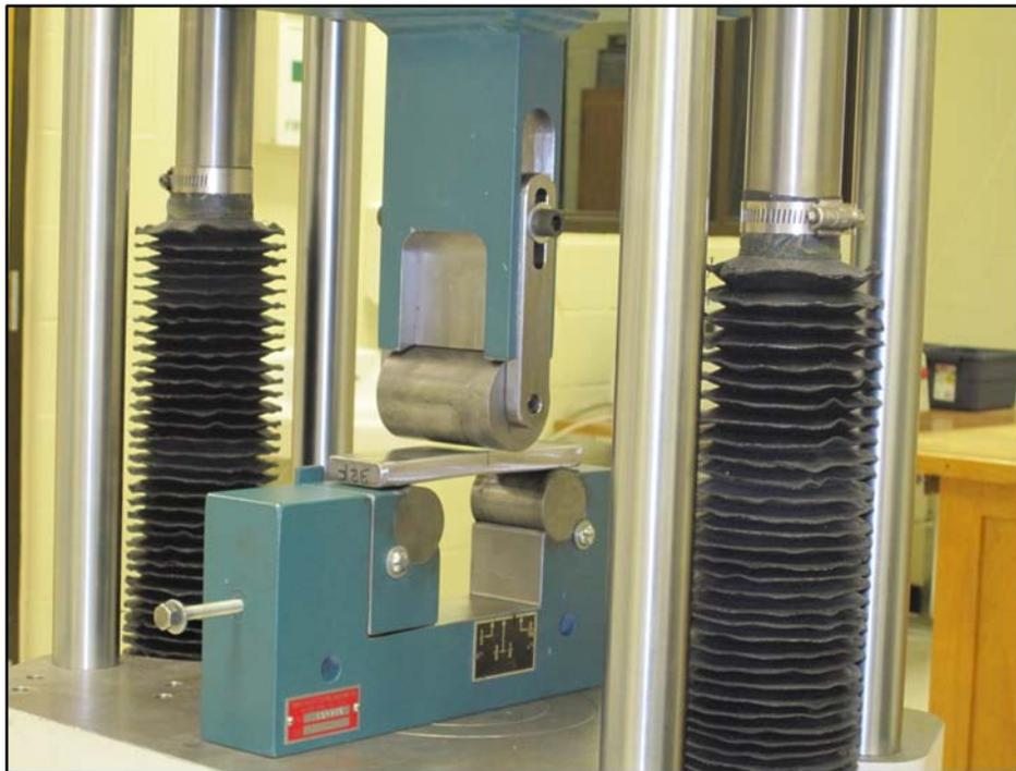
*Figure 13 Bottom Type Guided Bend Fixture with Test Specimen*
