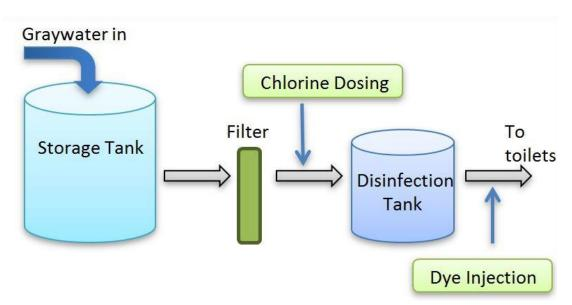
Figure 6.1 Graywater Treatment Process Schematic
