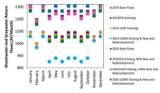
Figure 4.10 Impact to Return Flows for 25% Toilet Flushing, 75% Irrigation in 2014 and 2035
