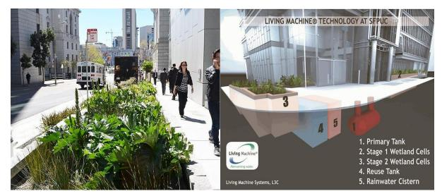
Figure 2.5 Photograph of Living Machine® Constructed Tidal Wetlands (left), Schematic of Living Machine® Technology (right) (Living Machine, 2012).
