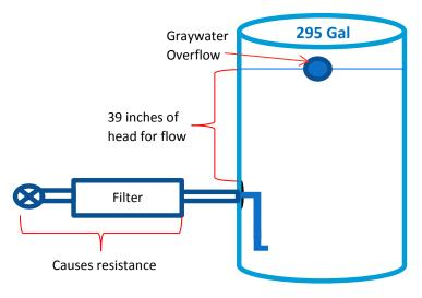
Figure 6.5 Schematic of Head Requirements in Graywater Storage Tank.
