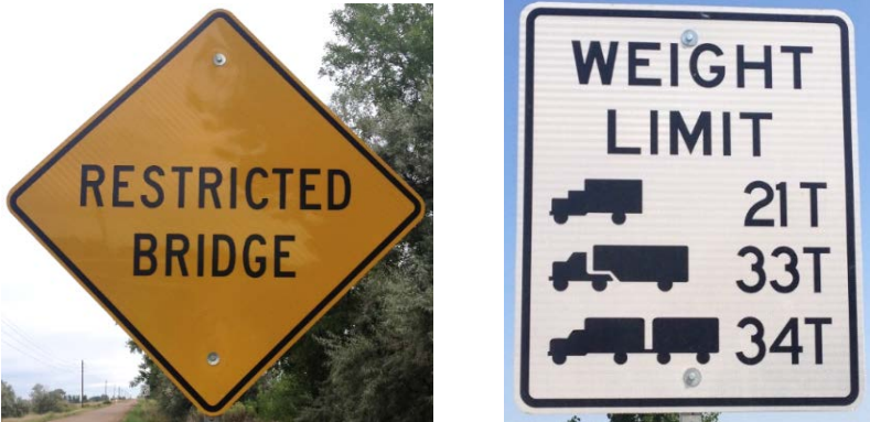
Figure 8.2 Advanced warning sign and load posting
