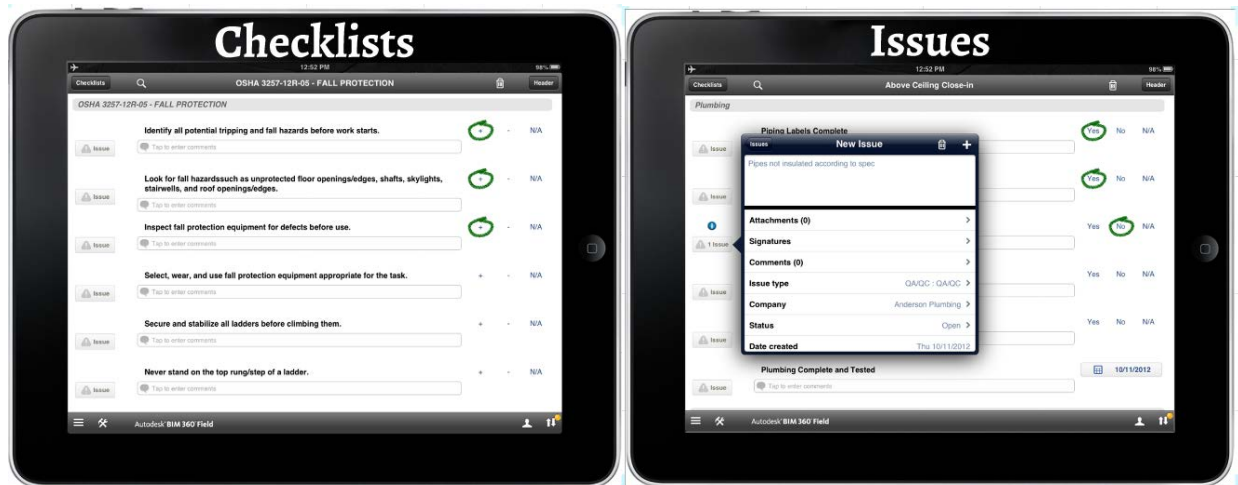
Figure 3.2 Left: BIM 360 Field inspection checklists. Right: BIM 360 Field issues in an inspection checklist. Photos from (Autodesk, 2014) [46]
