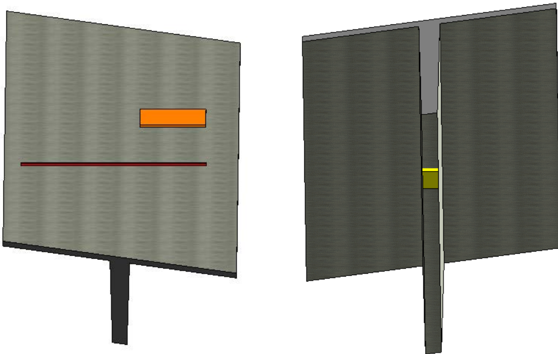
Figure 8.22 Left: view from top of Girder C with most severe cracking and delamination instances. Right: view from bottom of Girder C with most severe spalling instance
