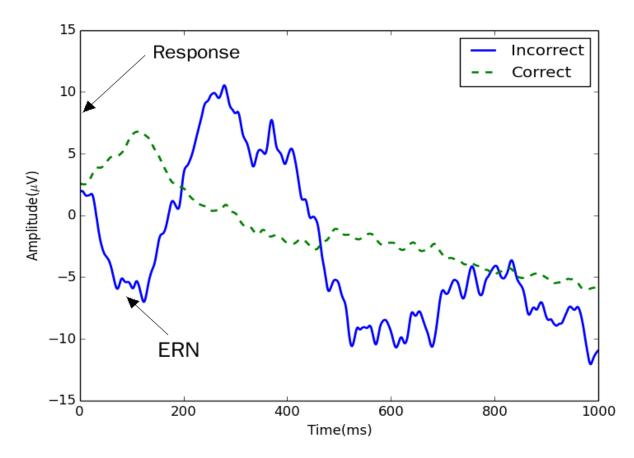
FIGURE 2.1. Average ERP for Subject 1 with correct and incorrect responses. The ERN is marked by a negative deflection around 50-100 ms after the response.
