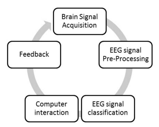
FIGURE 1.1. Common structure of a BCI system. The image is reproduced from [2].
