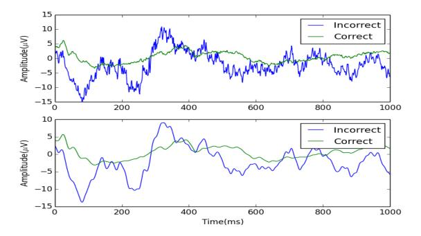
FIGURE 3.2. The average correct and incorrect responses for channel Cz before and after smoothing for Subject 2.
