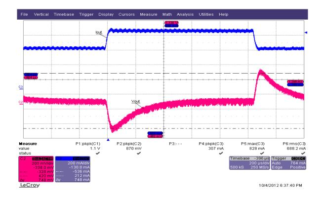
Figure 5.6 560mA to 800mA Load Transient response,  $V_{in}=3.5V V_{out}=12V$
