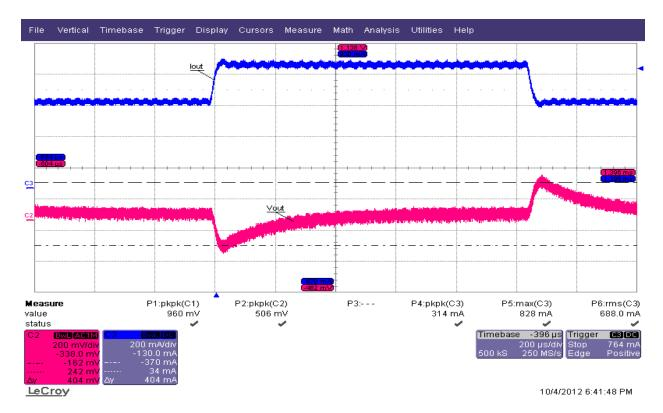
Figure 5.7 560mA to 800mA Load Transient response,  $V_{in}$ =5.5V  $V_{out}$ =12V
