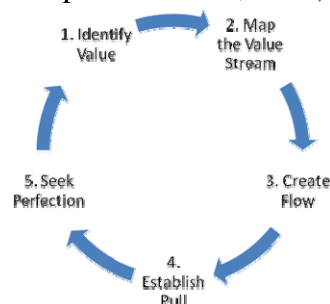
Figure 2.1. Flow chart demonstrating the five-step process for guiding the implementation of Lean Manufacturing techniques. Reprinted from “Principles of Lean” by Lean Enterprise Institute, 2009, http://www.lean.org/whatslean/principles.cfm . Copyright 2009 by Lean Enterprise Institute, Inc.
