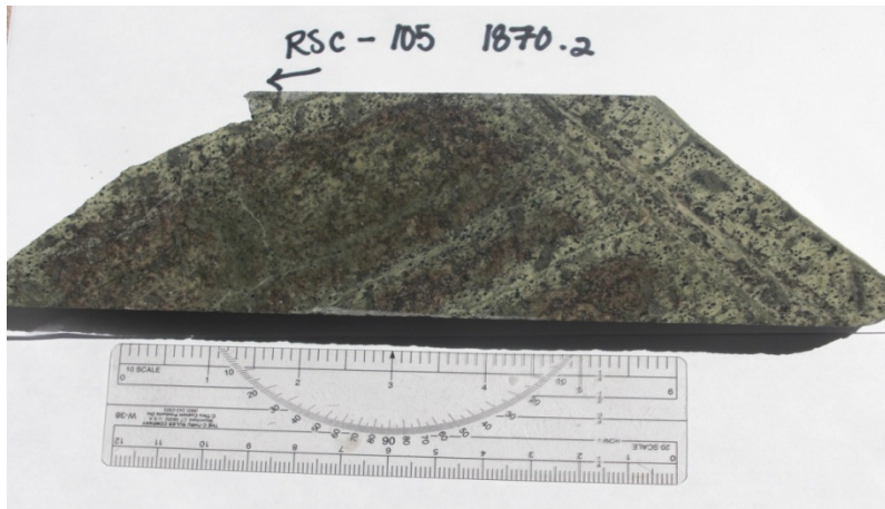
Figure 3.10 Photograph of phonolite showing potassic alteration (green color halo to calcite veins) from RSC-105 1870.2’.
