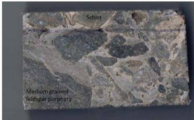
Figure 3.13 Handsample of porphyry+schist breccias with carbonate matrix from RSC-003 504.5'. The schist clasts have potassic alteration rims.
