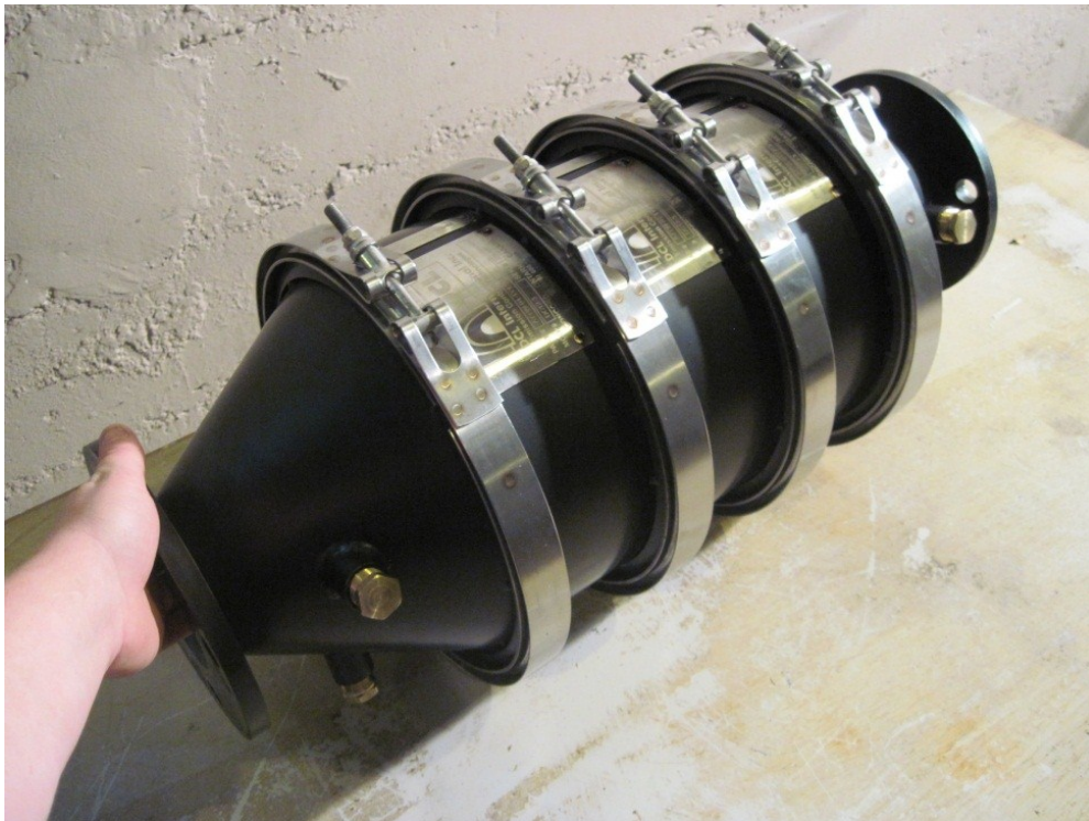
Figure 3-4: DCL International catalyst chosen for the project
