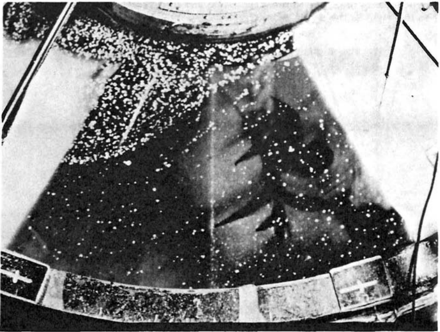
Fig. 18. Traces from dissolving dye crystals in a three-wave experiment with the 24.9 mm obstacle (050667). One of the waves can be seen in the upper left, where the aluminum particles have collected. In the eastern slope, a line of convergence is shown where westerly downslope flow meets easterly upslope flow. Experimental conditions are the same as in Fig. 11.
