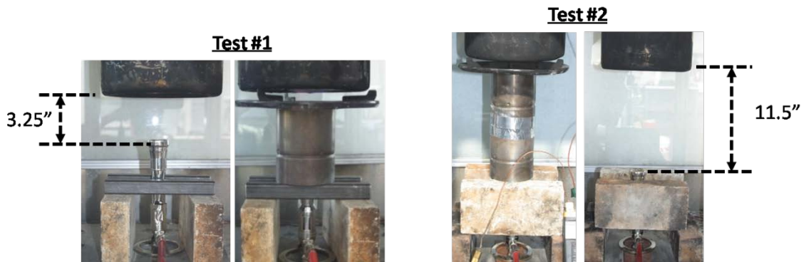
Figure 4.18. Pot configuration for tests #1 and #2.
