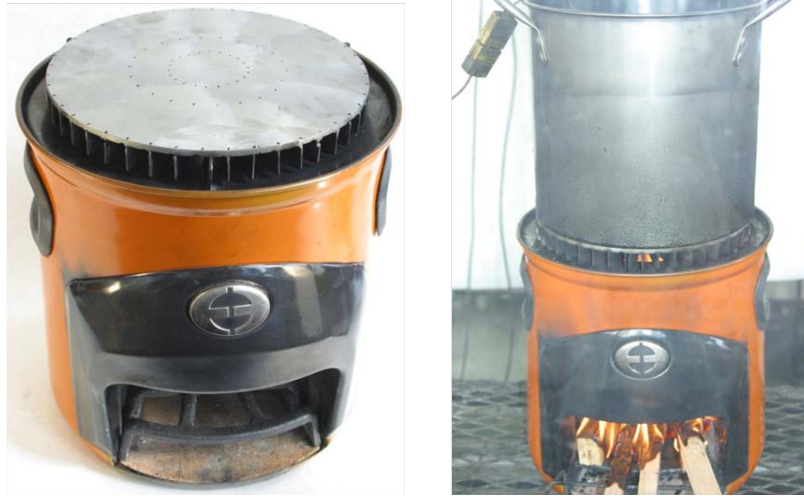
Figure 4.16. Images of the heat plate placed on top of the cookstove before and during testing.
