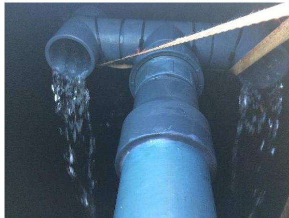
Figure 3.4: Planar schematic and picture of single inlet (left) & 4-way manifold inlet (right)
