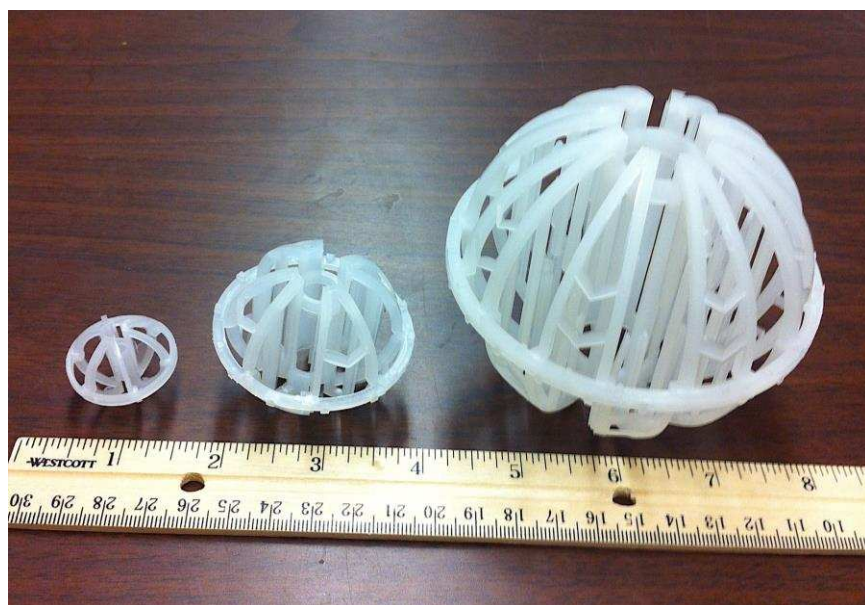
Figure 4.1: A photo of Jaeger Tri-Pack random packing material; 1” (Left), 2” (middle), and 3.5” (Right)
