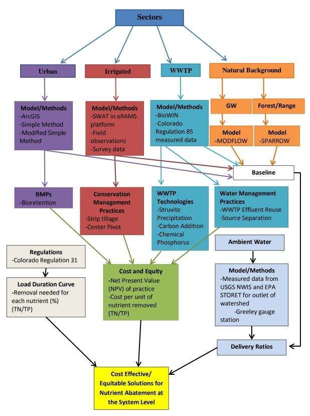
Figure 3.1: System Level Analysis Diagram of Cache la Poudre Watershed
