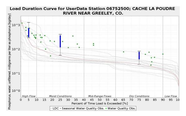
Figure 3.4: TP load duration curve for the Greeley, CO USGS Gauge Station based on Regulation 31 (warm water) river and stream standards for the years 2002-2015
