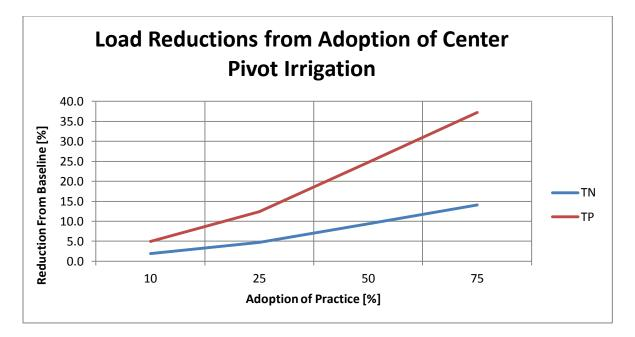
Figure 3.9: Percent nutrient load reductions from the baseline condition for center pivot irrigation adoption rates
