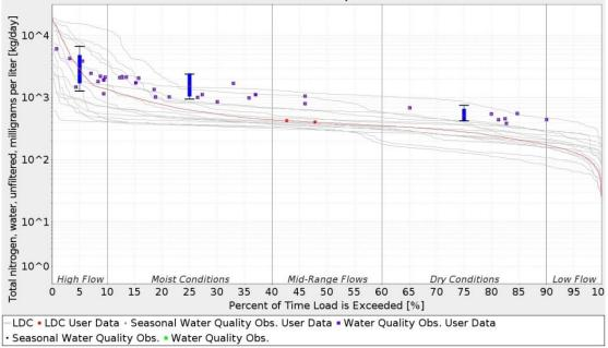
Figure 3.3: TN load duration curve for the Greeley, CO USGS Gauge Station based on Regulation 31 (warm water) river and stream standards for the years 2002-2015
